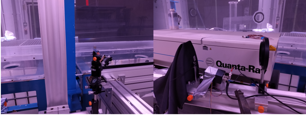
Figure 4.5: Setup to measure laser intensity. Left: A mirroring glass after the first regular mirror to reflect a very small part of the laser to the photo-diode. Right: The photo-diode in front of the laser head. Before the laser hits the photo-diode it travels through a polarizing filter
