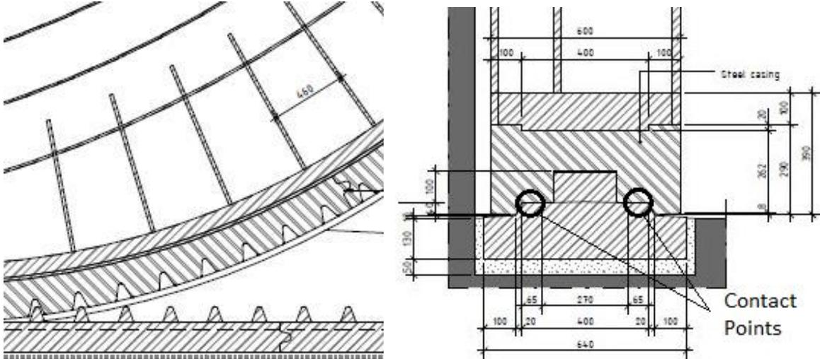
Figure 4-1 - Longitudinal and transversal cross section of the rail track
