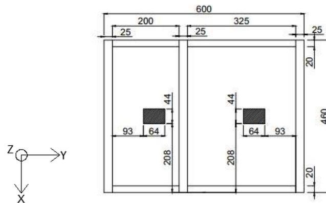
Figure 4-9 - Top view of the detail (shadow represents the locations of the forces)
