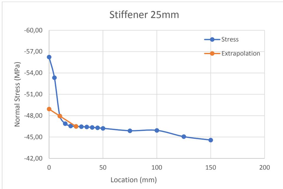
Figure 6-9 - Normal stresses on stiffener 2 and hot-spot extrapolation (Fine)
