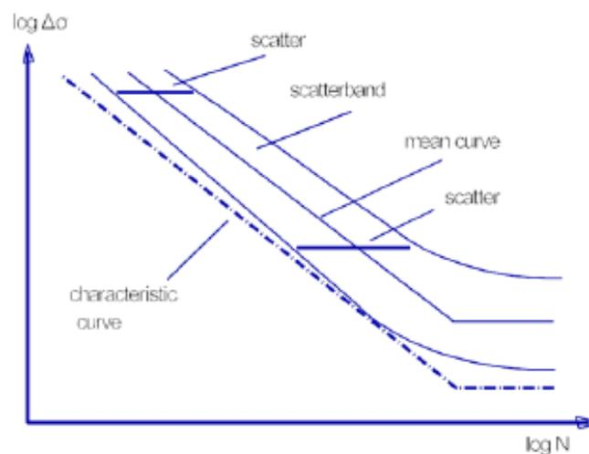
Figure 2-2 - S-N curve based on statistical evaluation for welds [15]
