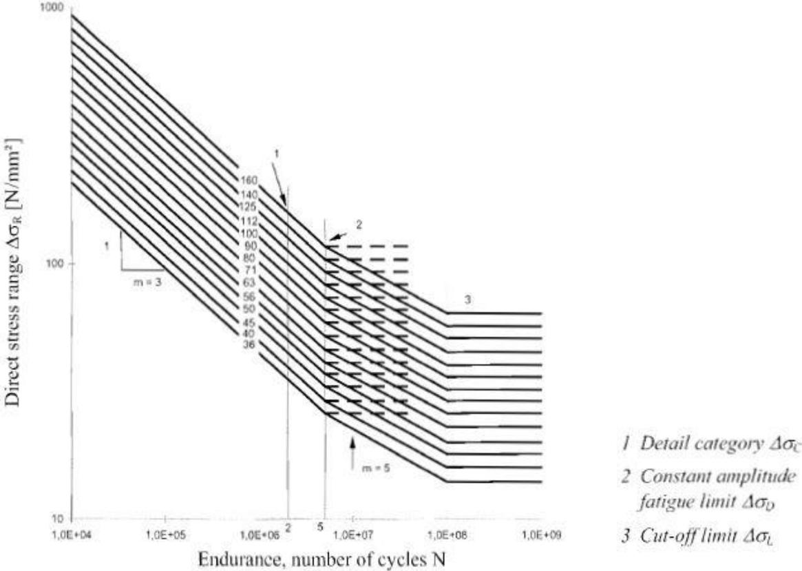
Figure 2-3 - Fatigue strength curves [10]
