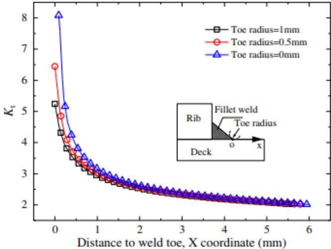
Figure 2-8 - Surface stress factor on the rib for different weld toe radius [26]
