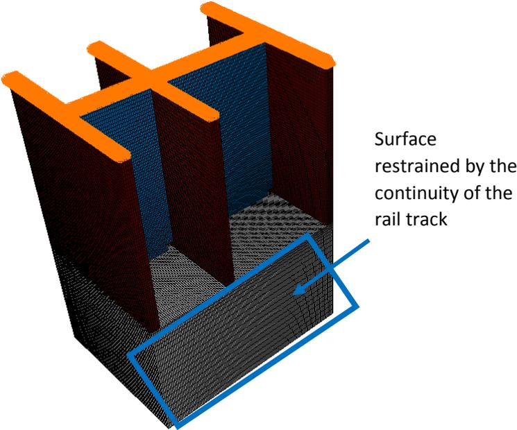
Figure 6-13 - Display of restrained surface on the local model
