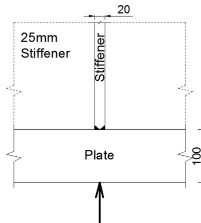
Figure 2-4 - Detail and measurements of plate and stiffener used in the bridge
