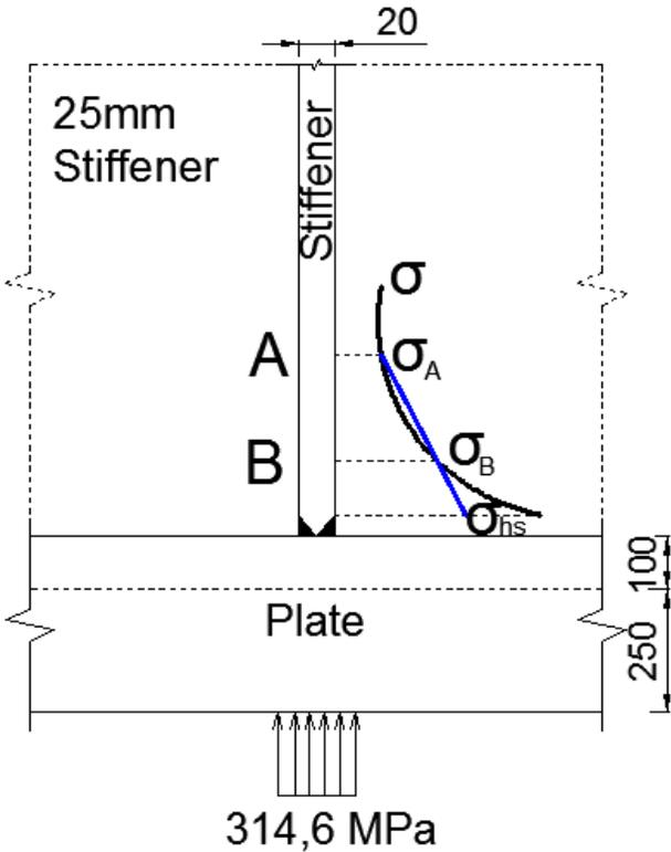
Figure 4-6 - Surface extrapolation of hot-spot stress from points A and B
