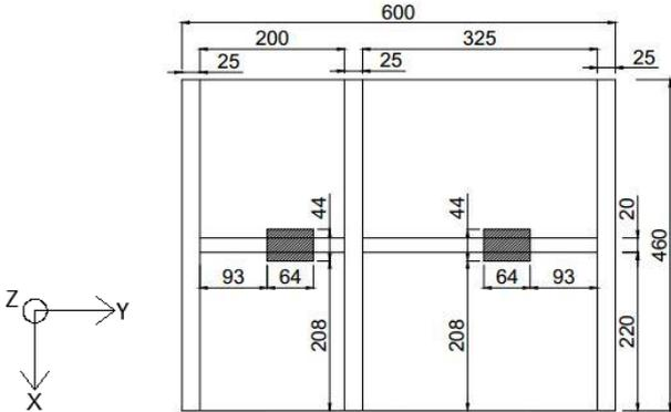
Figure 4-5 - Top view of the detail (shadow represents the locations of the forces)
