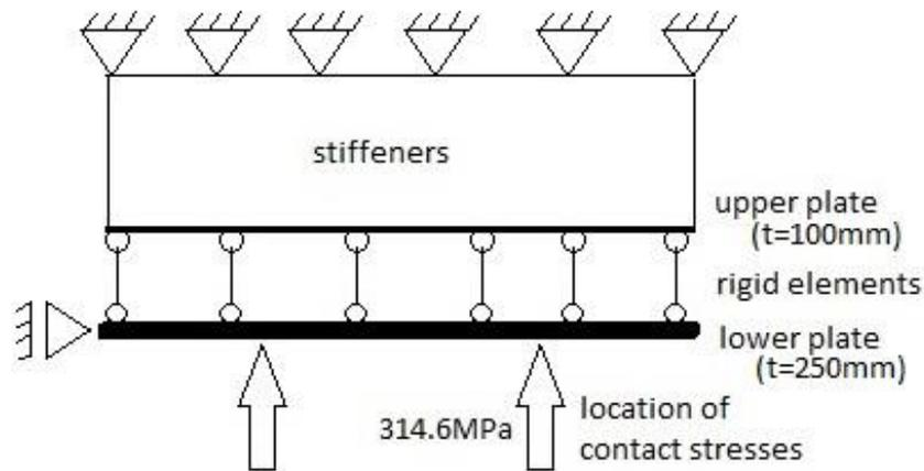
Figure 4-7 - Sketch of rigid elements that connect both plates together for the model
