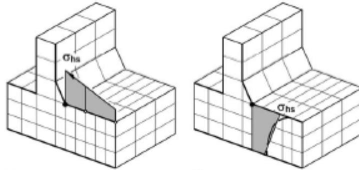
Figure 2-6 - Extrapolation at surface level (left) and through thickness (right) [12]
