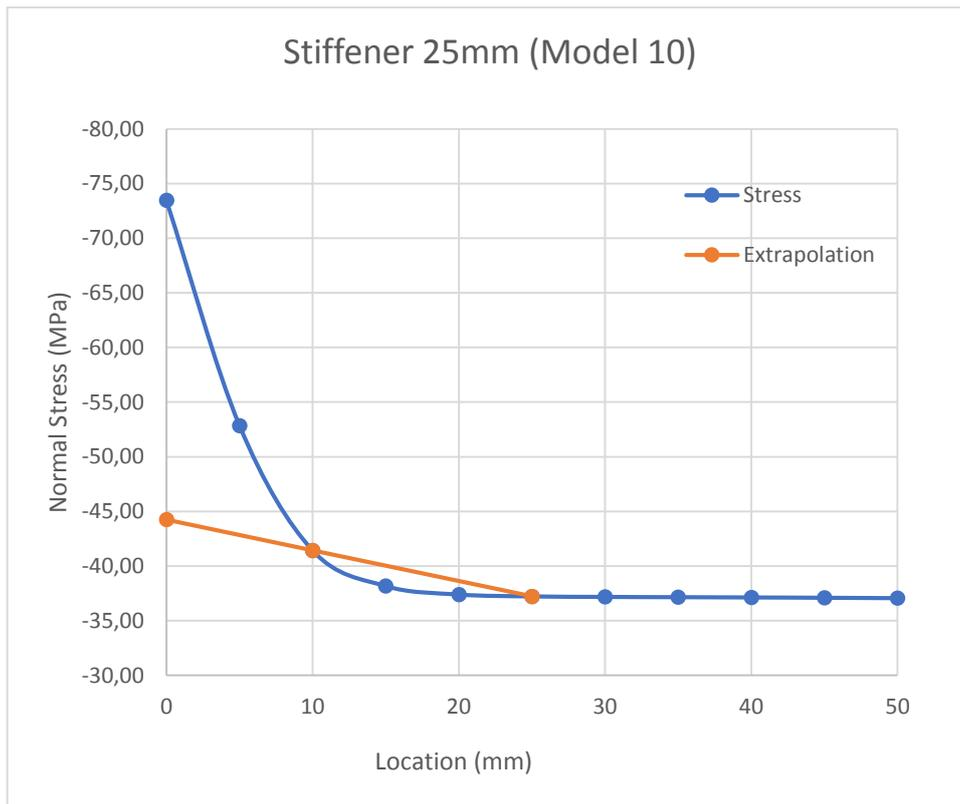
Figure 5-15 - Normal stresses on stiffener 2 and hot-spot extrapolation (Model 10)
