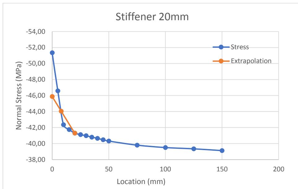
Figure 6-14 - Normal stresses on stiffener 1 and hot-spot extrapolation (Fine-weld)
