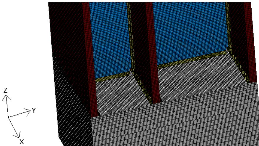
Figure 6-10 - Fillet weld modelling through solid elements (10mm weld – 45° angle)
