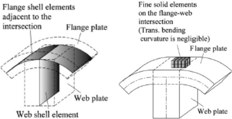
Figure 2-13 - Difference in curvature for shell and solid elements [21]
