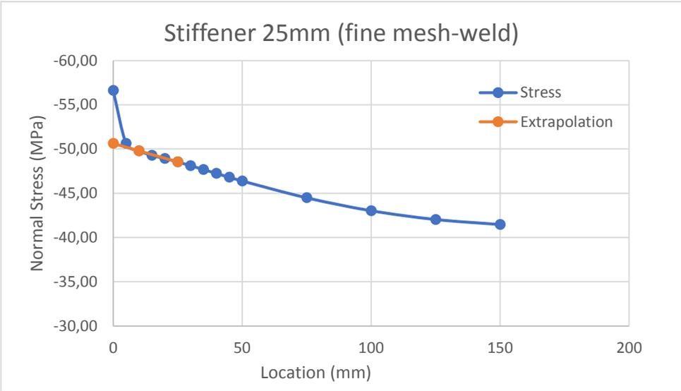
Figure 6-12 - Normal stresses on stiffener 2 and hot-spot extrapolation (Fine-weld)
