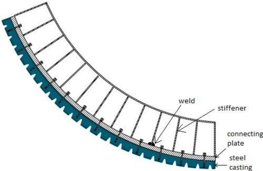
Figure 4-2 – Upper rail track where the plates and stiffeners are shown
