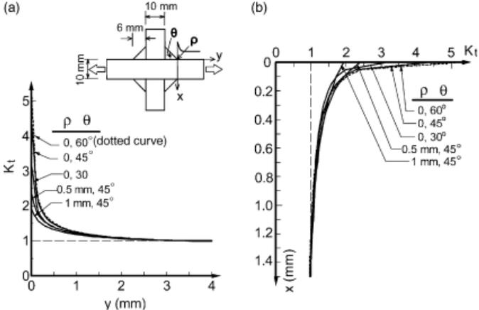
Figure 2-9 - Stresses distribution in weld toe region: (a) along surface; (b) through thickness [30]
