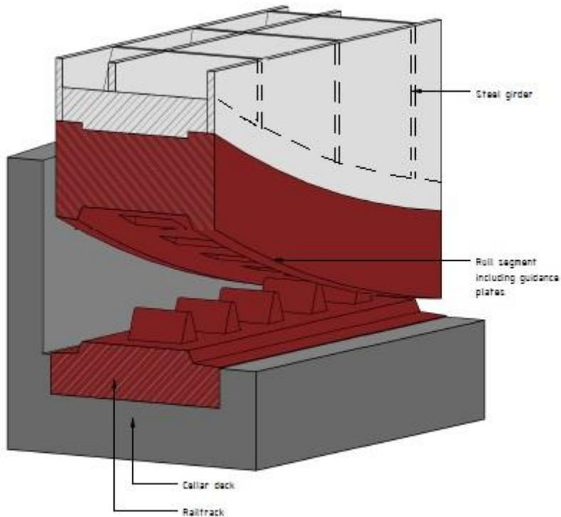
Figure 3-3 - 3D view of a section of the rail track
