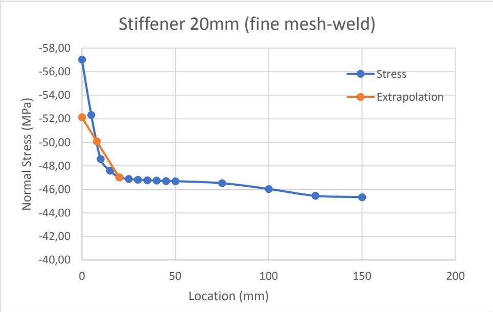
Figure 6-11 - Normal stresses on stiffener 1 and hot-spot extrapolation (Fine-weld)
