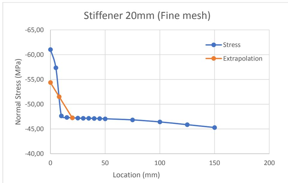
Figure 6-8 - Normal stresses on stiffener 1 and hot-spot extrapolation (Fine)
