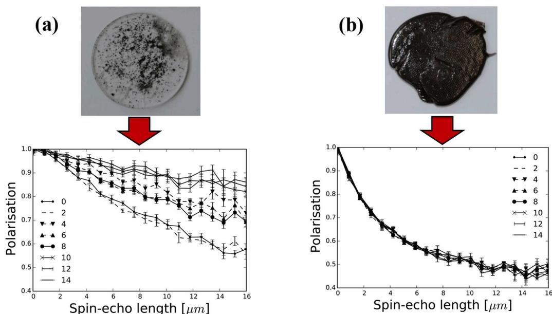
Fig. 3. SESANS scans in 2 mm steps across the samples of (a) unprocessed sample with 3.0 wt% C<sub>60</sub>; (b) sample with 5.0 wt% C<sub>60</sub> collected from P9 (rate = 130 g/h).
