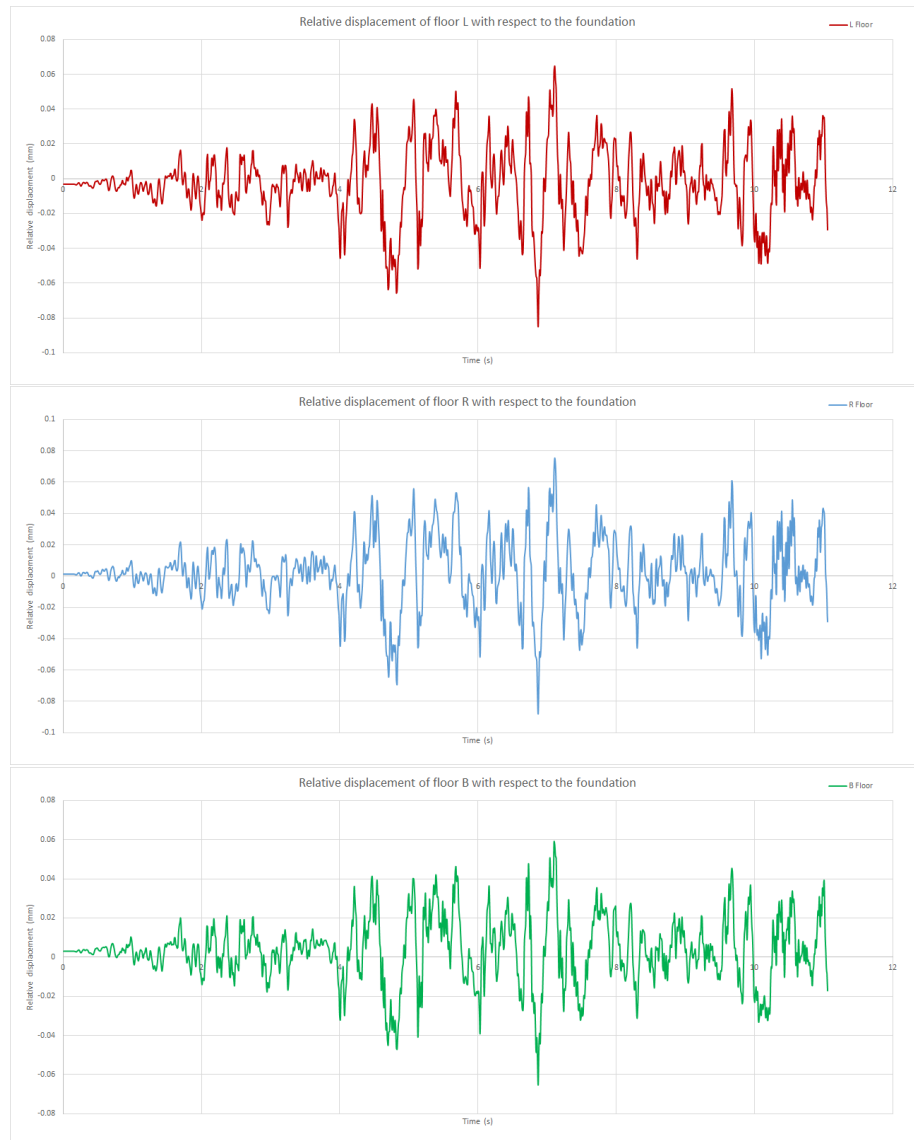
Figure 5-67: Relative displacement of the floors L,R and B with reference to foundation
