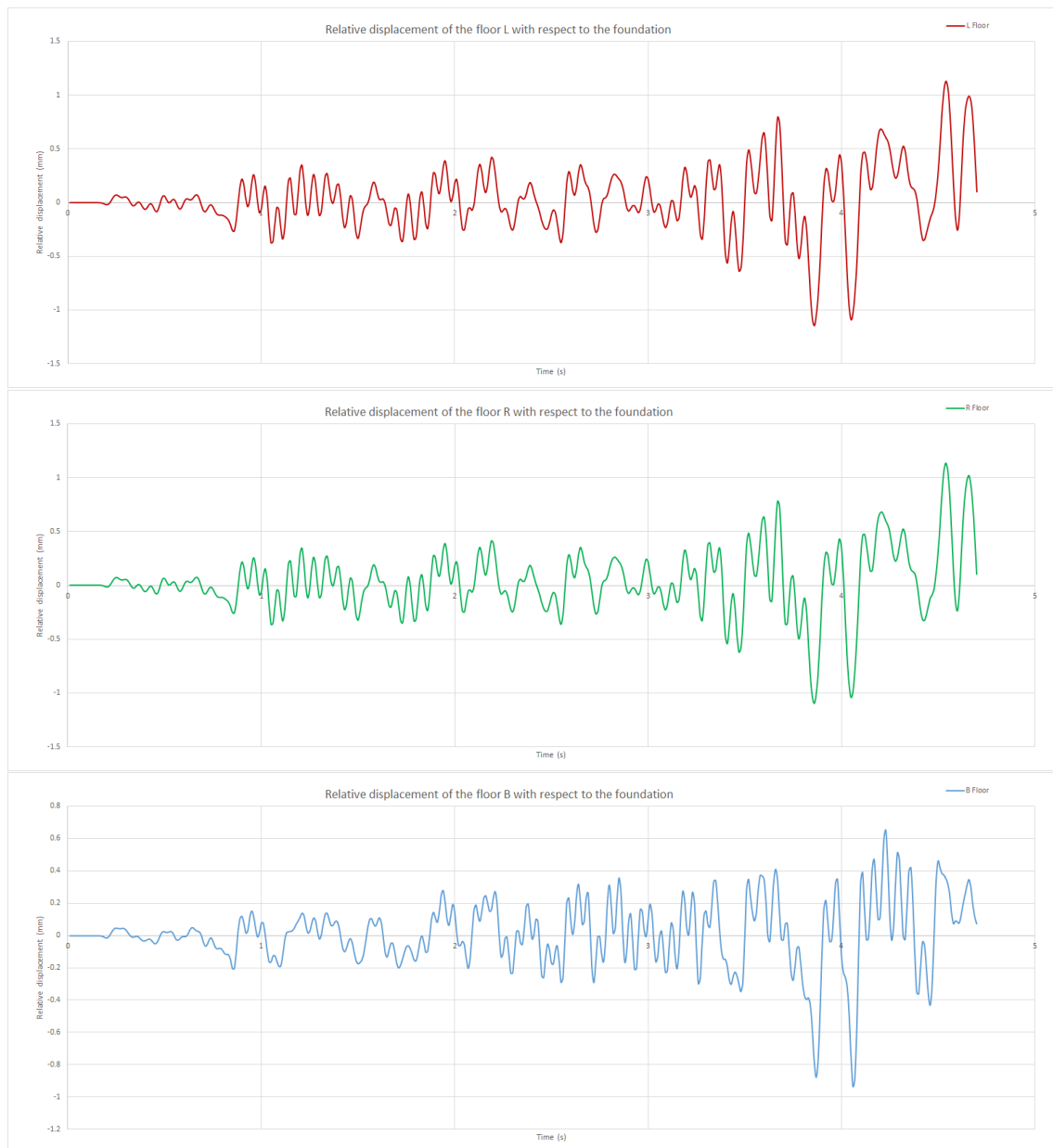
Figure 5-16: Relative displacement of the floors L,R and B with reference to foundation
