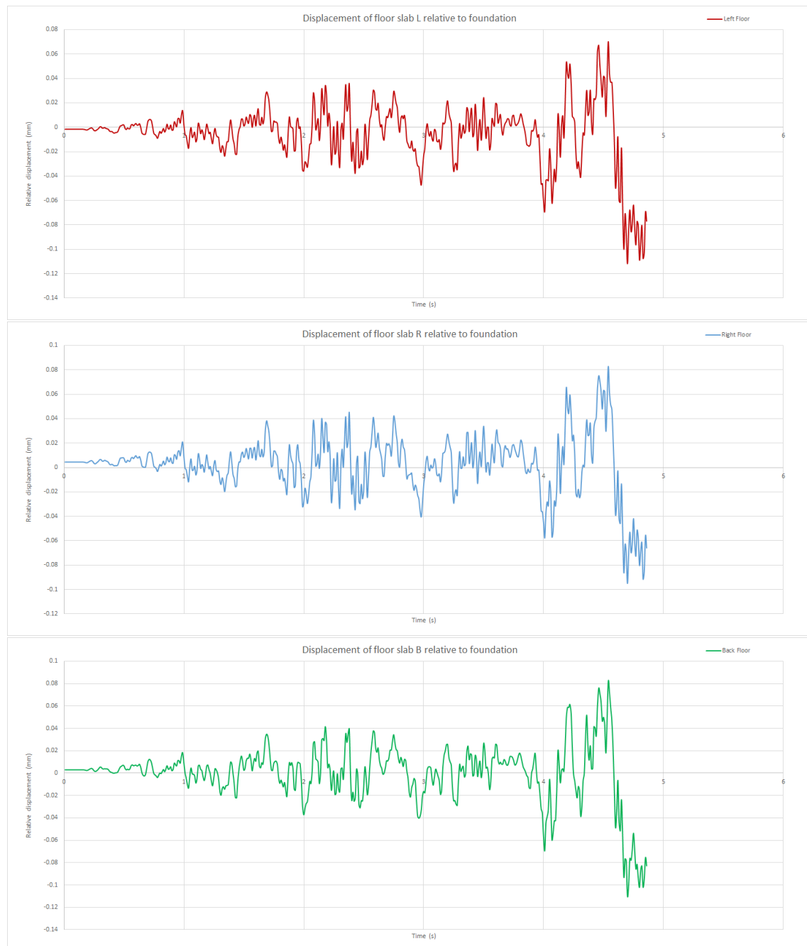
Figure 5-36: Relative displacement of the floors L,R and B with reference to foundation
