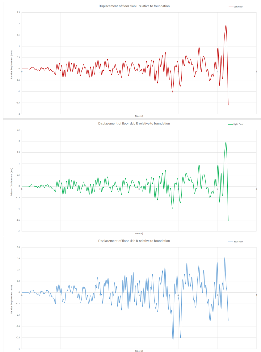
Figure 5-18: Relative displacement of the floors L,R and B with reference to foundation
