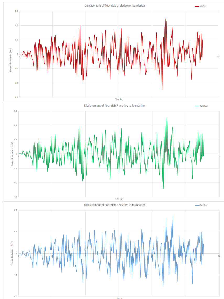
Figure 5-8: Relative displacement of the floors L,R and B with reference to foundation
