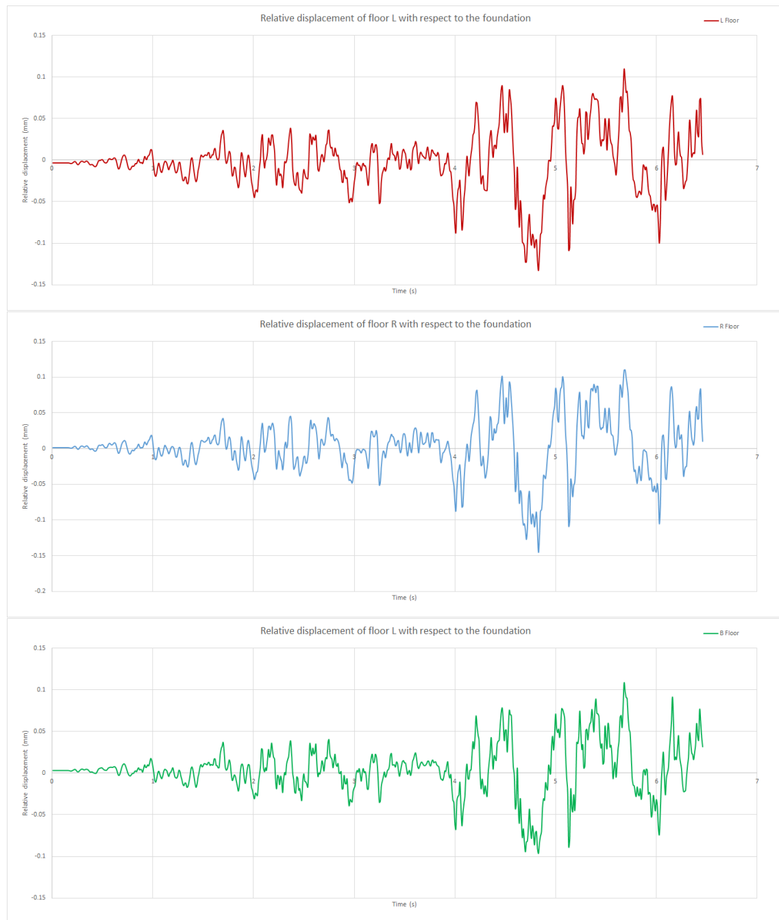
Figure 5-77: Relative displacement of the floors L,R and B with reference to foundation
