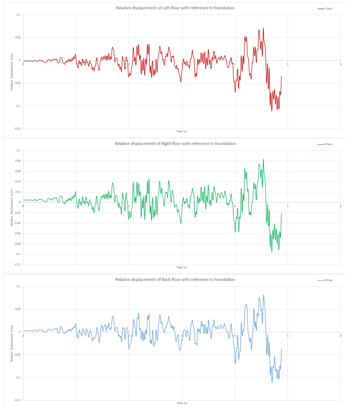
Figure 5-33: Relative displacement of the floors L,R and B with reference to foundation
