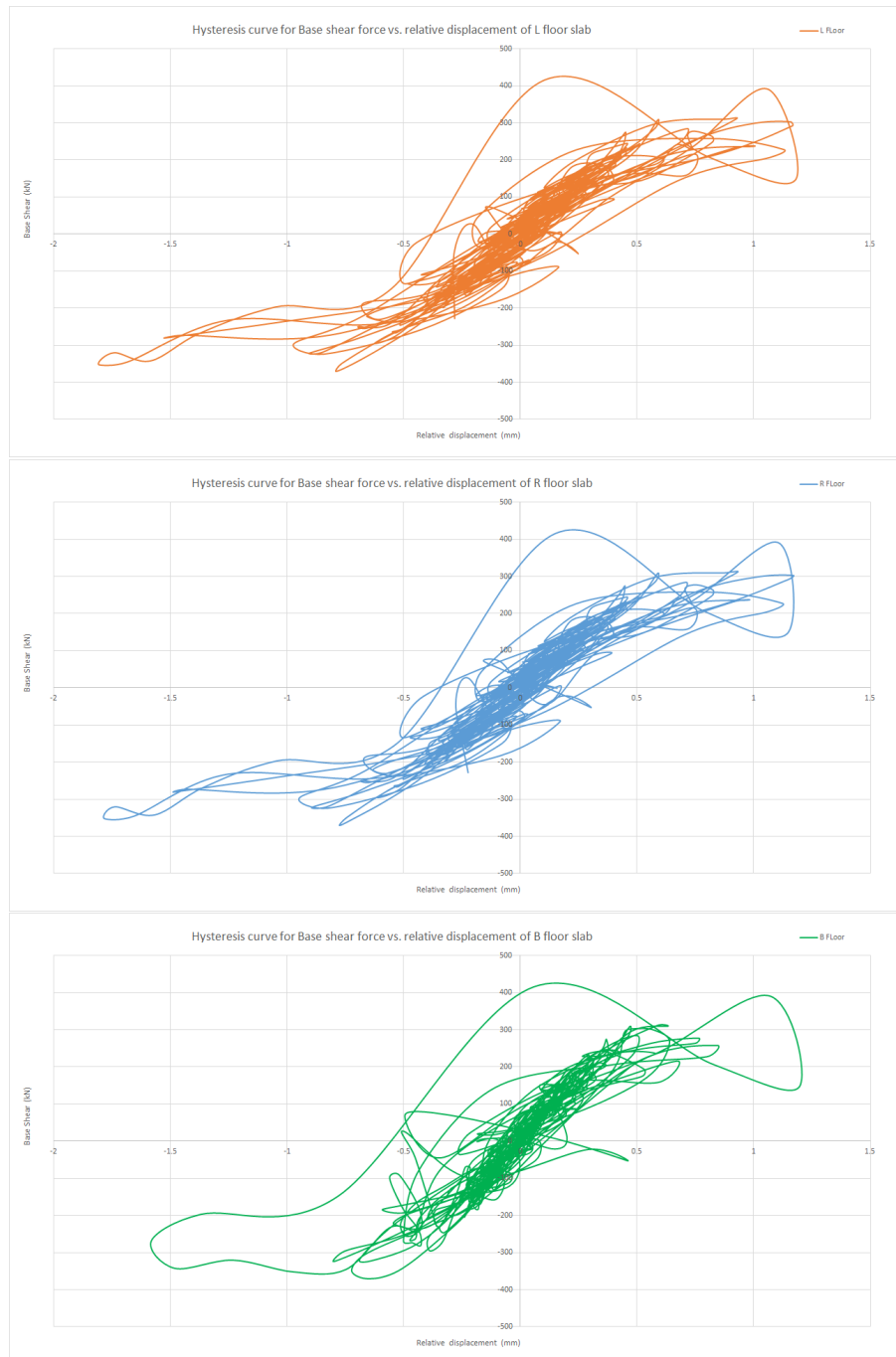
Figure 5-55: Hysteresis curve for base shear vs. relative displacement of the floors L,R and B with reference to foundation
