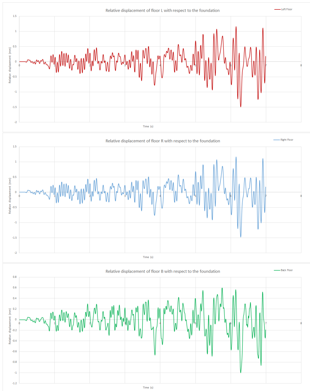
Figure 5-57: Relative displacement of the floors L,R and B with reference to foundation
