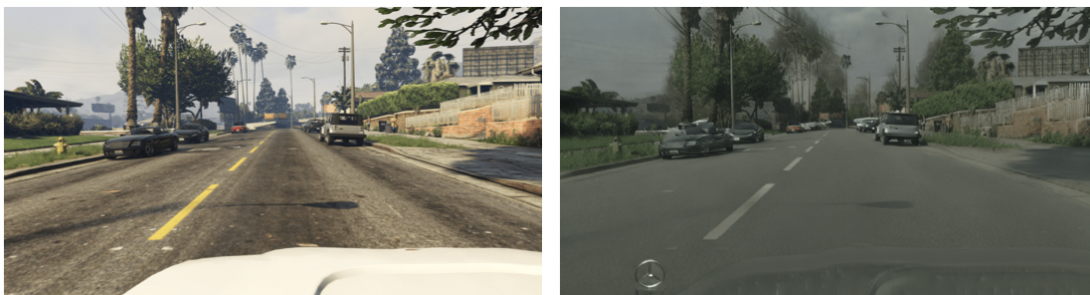
Figure 5: CyCada Domain Adaptation takes a synthetic image and outputs the same image with similar domain to a real world image. Image taken from: Hoffman et al. (2018)
