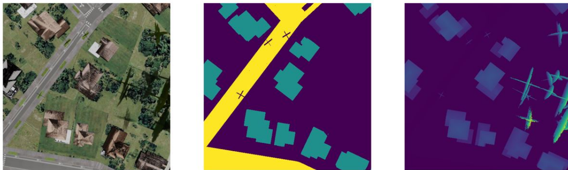
Figure 9: Left: Color image from synthetic city. Centre: Semantic segmentation of the image. Right: DSM of the synthetic city.
