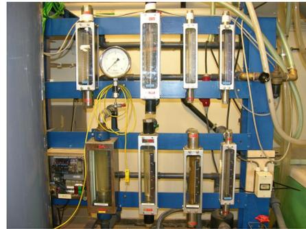
(b) Image of the set of rotameters which are used to measure the flow rates of both the gas (upper row) and liquid phase (lower row). The overlapping ranges allow accurate measurements in all regimes.
