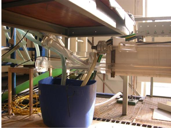
**Figure 3.5:** Image of the inlet type 'b' installed in the set-up. The liquid comes in horizontally, the gas from above. After the inlet, which is 1 m in length, both phases flow parallel because of the separator plate that is installed inside the tube.
