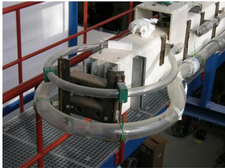
(a) Image of the turning point halfway the set-up. The radius of the turn is large compared to the diameter of the pipe ( $R/D = 6$ ), so the effect on the flow is limited. Within 2-5 m after the turn, the effect has completely vanished.
