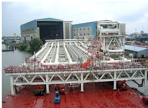
**Figure 1.7:** Large slug catcher, the equipment measures 140 by 36 meters.
