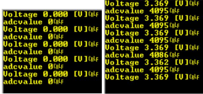
(a) Output at an input of 59mV (b) Output at an input of 3.369V
