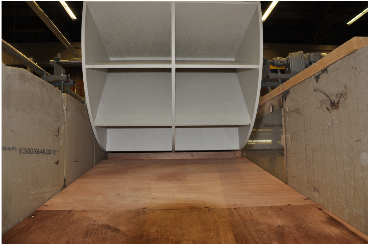
Figure A.10: Connection between crest element and paddle wheel, the losses are minimized
