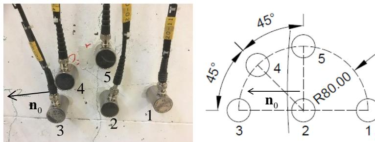
Figure 4.17: Sensor arrangement with the transducer in the middle and the receivers around
