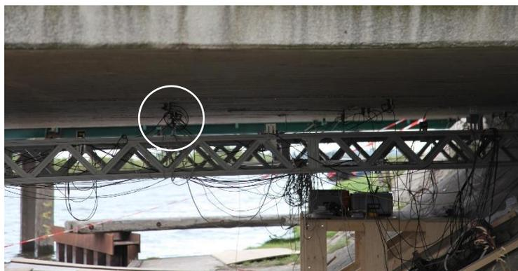
*Figure 1.1: AE tests on Ruytenschildt bridge*
