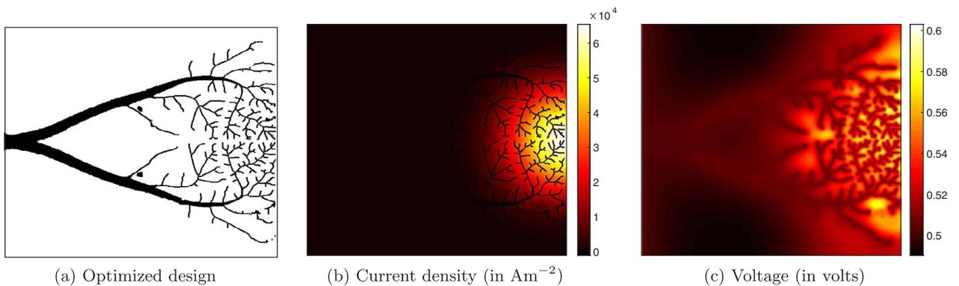
Fig. 14. Optimized design and the current density and voltage distributions for the front side of a solar cell under a Gaussian illumination of an average intensity of 12 suns ( $A_0 = 15$ ) and a Gaussian temperature profile with base temperature of 320 K and temperature amplitude equal to 40 K. The optimal busbar potential  $V_b$  and efficiency  $\eta$  values are 0.503 volts and 15.033%, respectively.
