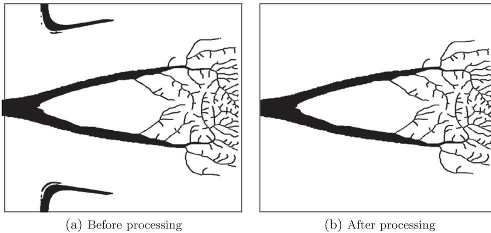
**Fig. 12.** Optimized design obtained using topology optimization (left), and its post-processed version (right) for the front side of a solar cell under a Gaussian illumination of an average intensity of 12 suns ( $A_0 = 20$ ). The post-processing removed electrode material that remained in dark regions of the cell.
