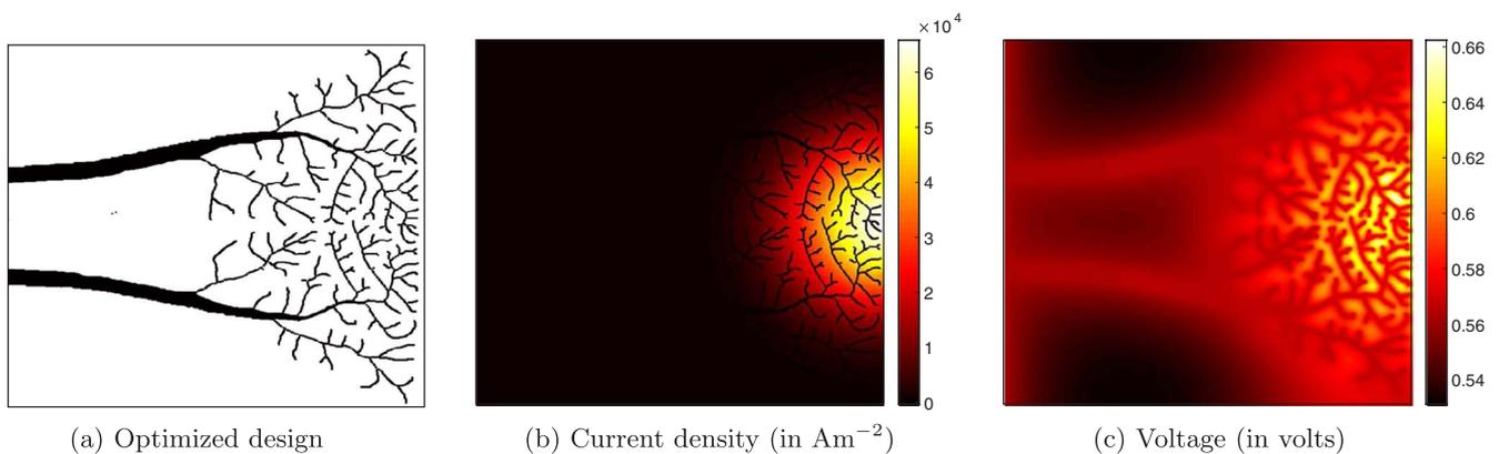
Fig. 10. Optimized design and the current density and voltage distributions for the front side of a solar cell under a Gaussian illumination of an average intensity of 12 suns ( $A_0 = 15$ ). A uniform temperature profile is chosen with base temperature set to 320 K. The optimal busbar potential  $V_b$  and efficiency  $\eta$  values are 0.562 volts and 17.271%, respectively.
