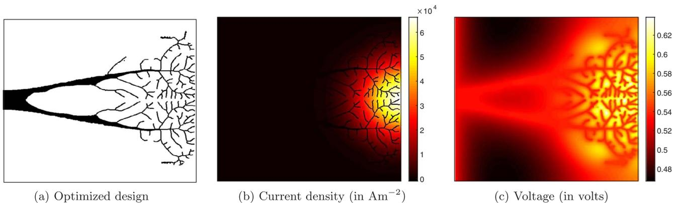
Fig. 15. Optimized design and the current density and voltage distributions for the front side of a solar cell under a Gaussian illumination of an average intensity of 12 suns ( $A_0 = 15$ ) and an anti-Gaussian temperature profile with base temperature of 320 K and temperature amplitude equal to 40 K. The optimal busbar potential  $V_b$  and efficiency  $\eta$  values are 0.532 volts and 16.271%, respectively.
