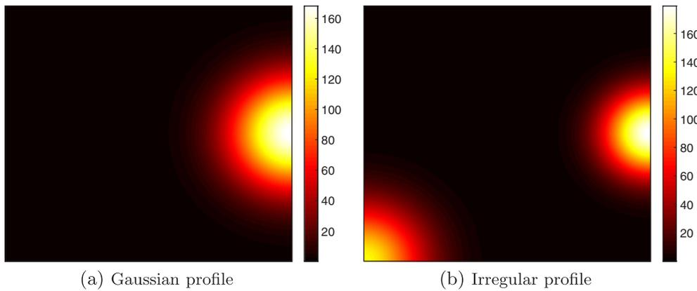
Fig. 7. Non-uniform illumination profiles with an average illumination of 12 suns (1 sun =  $1000 \text{ W m}^{-2}$ ). For the Gaussian profile,  $A_0$  is equal to 15 and for the irregular profile  $A_0$  values are 15 and 20 for the two Gaussian distributions.
