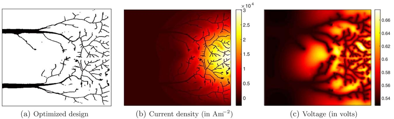
Fig. 9. Optimized design and the current density and voltage distributions for the front side of a solar cell under a Gaussian illumination of an average intensity of 12 suns ( $A_0 = 10$ ). A uniform temperature profile is chosen with base temperature set to 320 K. The optimal busbar potential  $V_b$  and efficiency  $\eta$  values are 0.535 volts and 17.075%, respectively.
