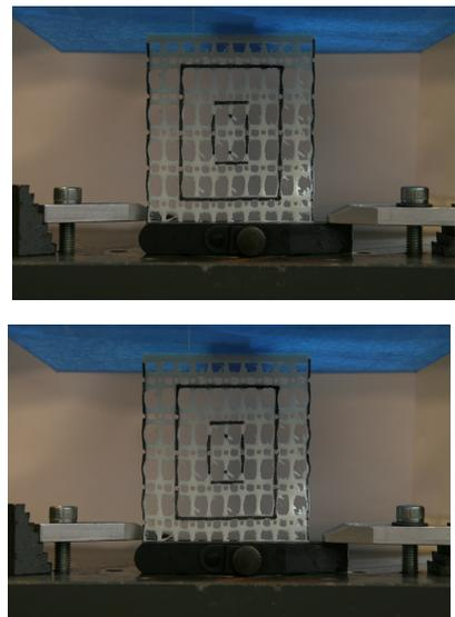
Poisson's values and deformed configuration for design ID5
