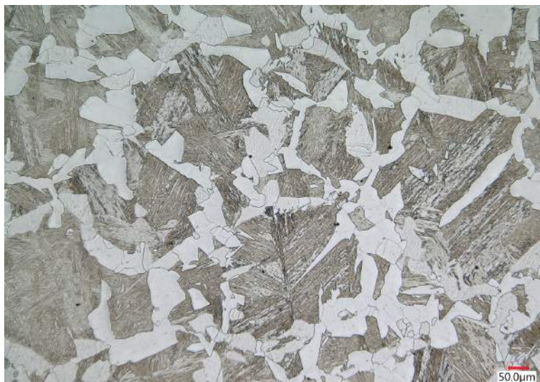
Figure 3.12: Optical image, magnification 250x, of dual-phase sample DP2, annealed at 700°C for 15 minutes; scale bar: 50 \mu m
