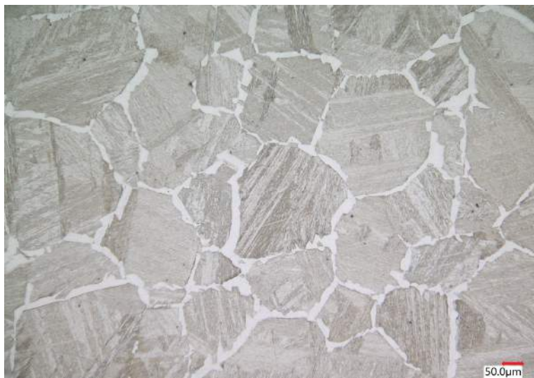
Figure 3.14: Optical image, magnification 250x, of dual-phase sample DP4, annealed at 700°C for 3 minutes; scale bar: 50 μm
