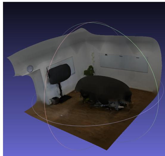
(b) Reconstructed mesh model of office point cloud
