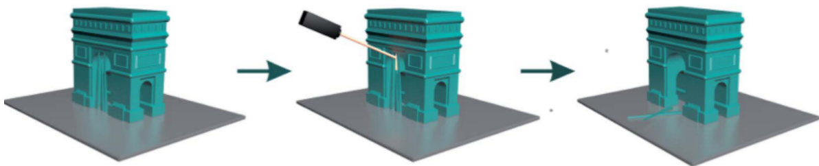
Figure 2.6: Support structures can be precisely removed by locally applying laser induced heat. Reproduced from [34].
