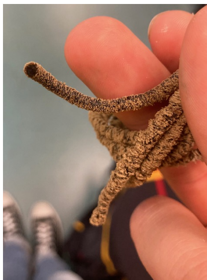
Figure E.2: The extrudate burned after a longer residence time in which the network reduced in dynamic properties during a second extrusion cycle at 200 °C.
