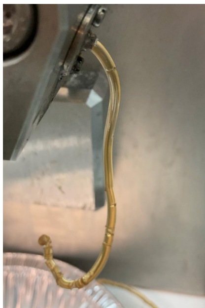
Figure E.1: The extrudate turns more yellow and small cracks start to appear due to a longer residence time at 200 °C in the extruder.
