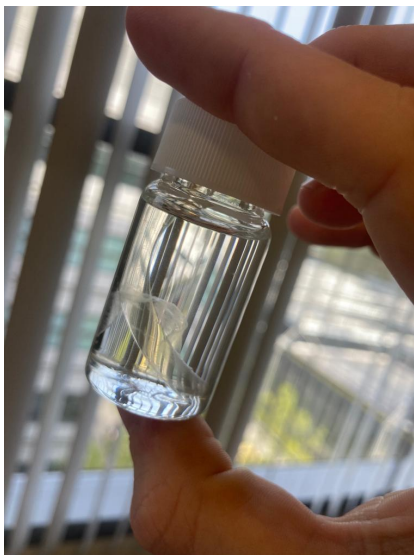
Figure E.4: Extrudate swollen for 24 hours in THF.
