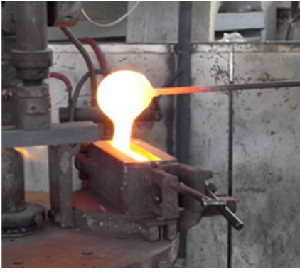
Figure 57: The process of casting glass. Glass is poured into the mould.
