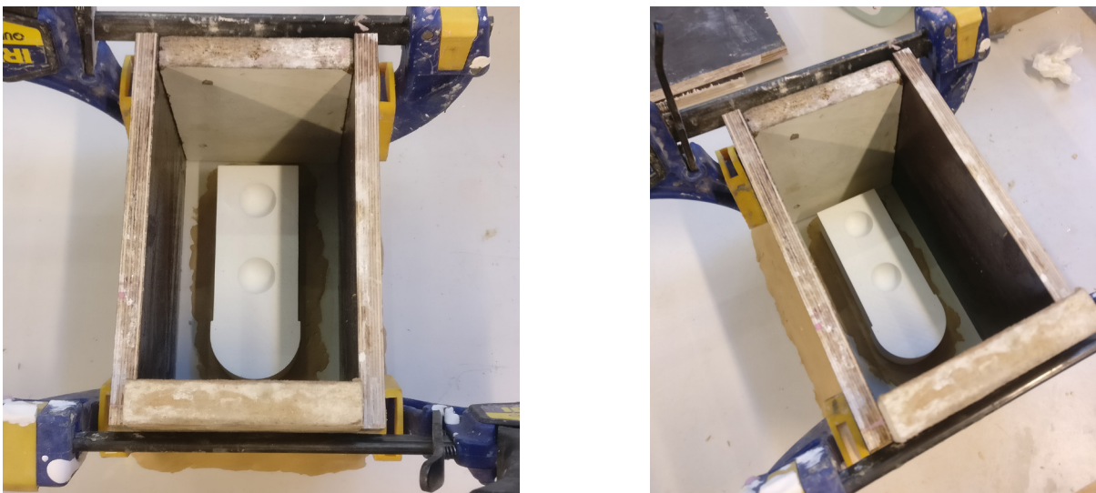
Figure 170: Preparation of the silicon mould.
