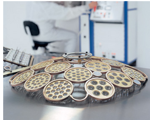
Figure 94 : Vacuum chamber and planetary optic holder
