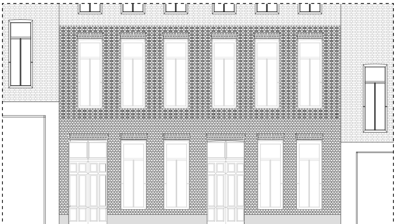
Figure 162: New elevation with the new components in the upper part of the glass facade
