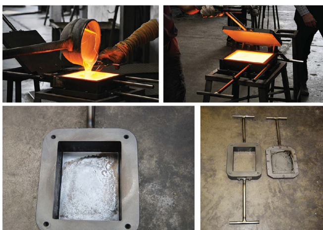
Figure 73: The casting of the soda-lime glass blocks.
