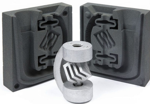
Figure 163 : 3D printed sand mould (left), high precision mould.
