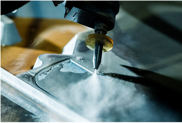
Figure 29 : Water jet cutting method.
