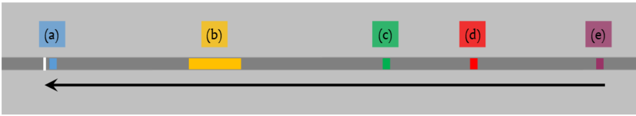
Figure 5-2 | Detection configuration according to the IVER 2002 guidelines, given by Siteur, et al. (2002), with the stop line detector (a), followed by the long detector (b), and three distant detectors (c), (d), and (e).
