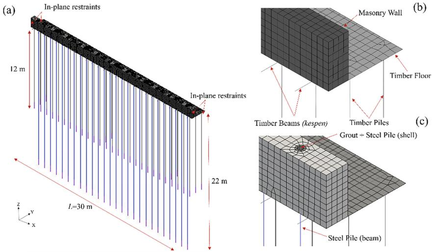
**Fig. 4.** Numerical model adopted to assess the response of *Marnixkade* under traffic loading: (a) general isometric view of the strengthened model; (b) close-up of the general isometric view of the unstrengthened model; (c) close-up of the general isometric view of the strengthened model.
