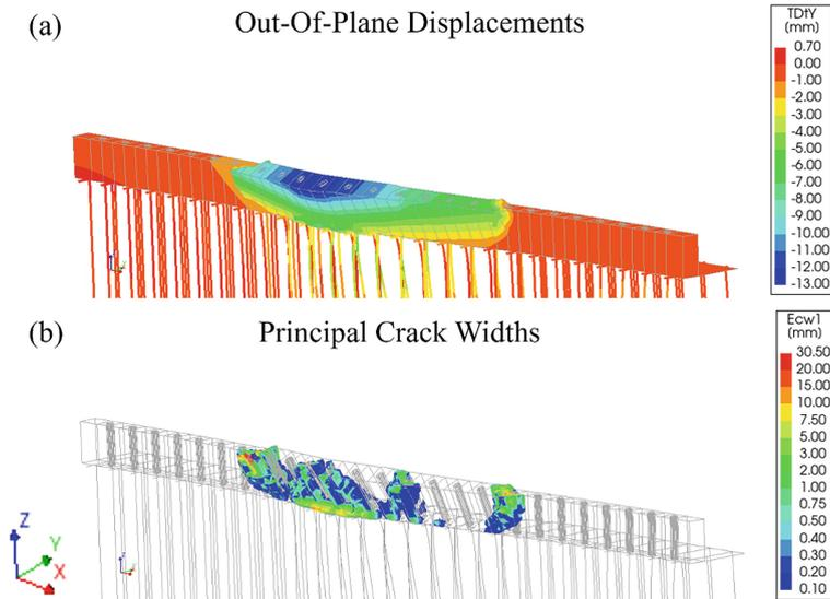
**Fig. 10.** Failure mechanism in the strengthened numerical model at  $LM = 79$  in terms of: (a) out-of-plane displacements and (b) principal crack widths (Deformation Scale Factor = 100).
