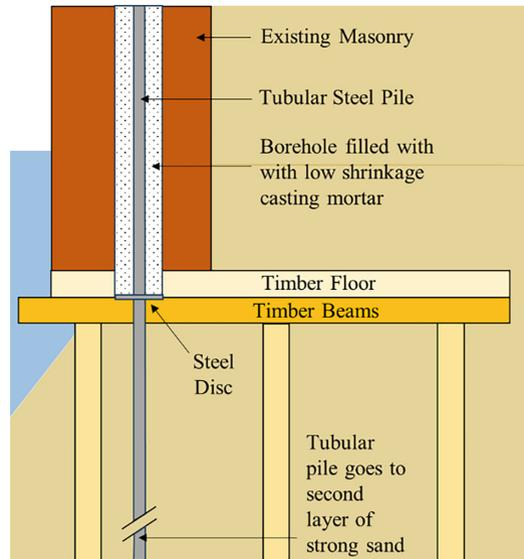
**Fig. 2.** Schematic of the assessed strengthening technique.
