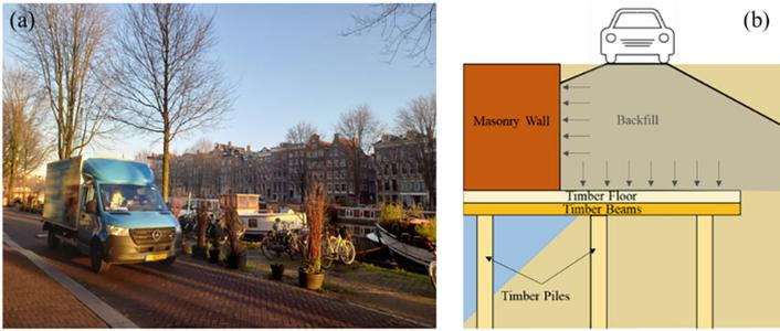
**Fig. 1.** (a) Vehicular traffic on carriageways constructed on the backfill of masonry quay walls in Amsterdam, the Netherlands and (b) schematic showing how this vehicular traffic creates pressure distributed by the soil on quay wall structures.
