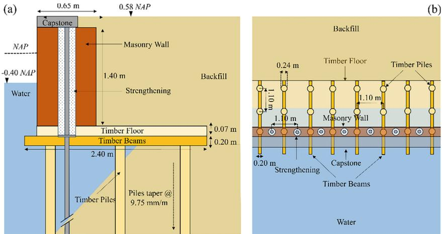
**Fig. 3.** Geometry of *Marnixkade* assumed for the numerical model with strengthening features inserted: (a) transversal cross-section and (b) plan view.
