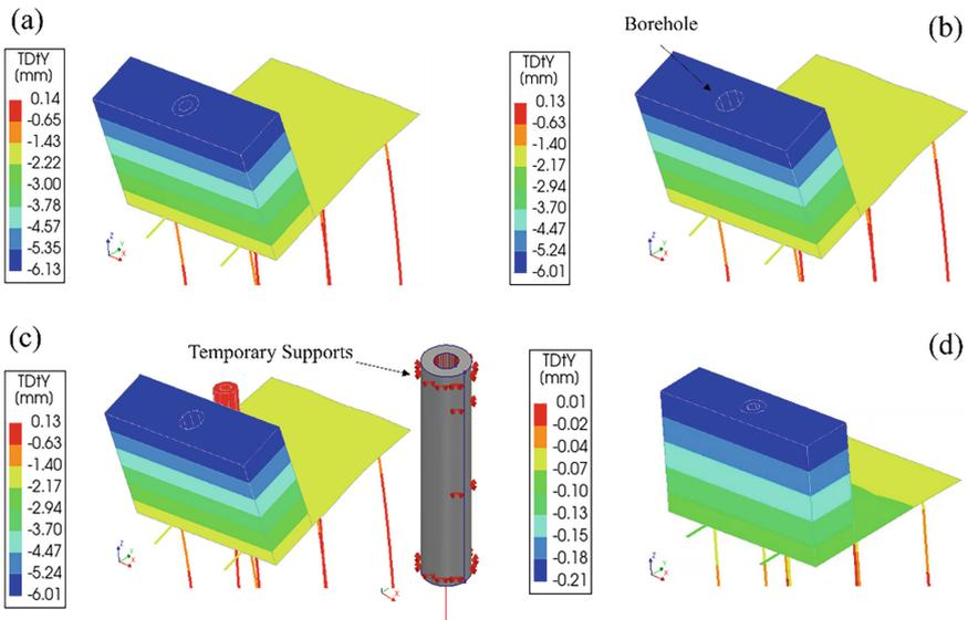
**Fig. 6.** Phased Analysis for simulation of the installation of the strengthening technique: (a) initial application of dead load and soil and water pressure; (b) simulation of borehole drilling for the tubular steel pile; (c) temporary support of the tubular steel pile within the model before establishing connections and (d) clear displacements in the model, finalise connection between the tubular steel pile and the masonry and apply parking load (Deformation Scale Factor = 100).
