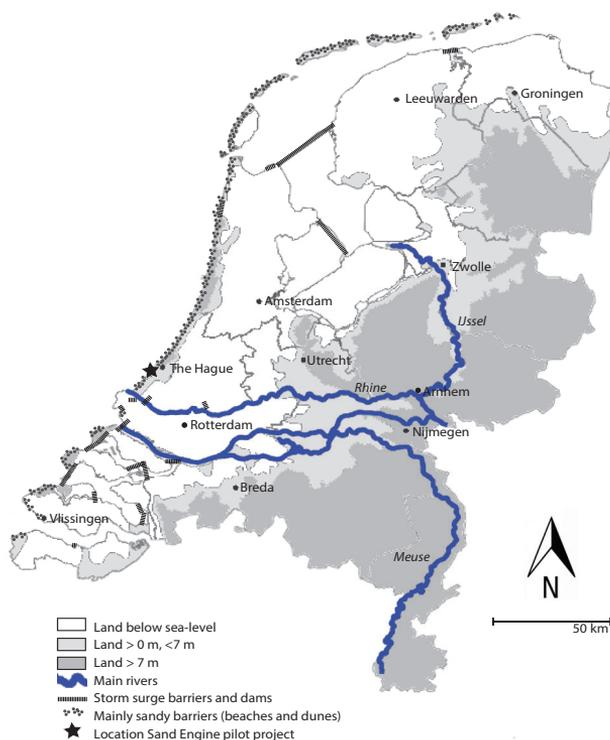
Figure A-2. Map of the Netherlands, showing the parts below and around sea level, its main rivers, the main hard coastal defence infrastructures (storm surge barriers and dams), the sandy coastal defence structures and the location of the Sand Engine pilot project. Map adapted from Van der Maarel (2010), based on Van der Bolt et al. (2010).
