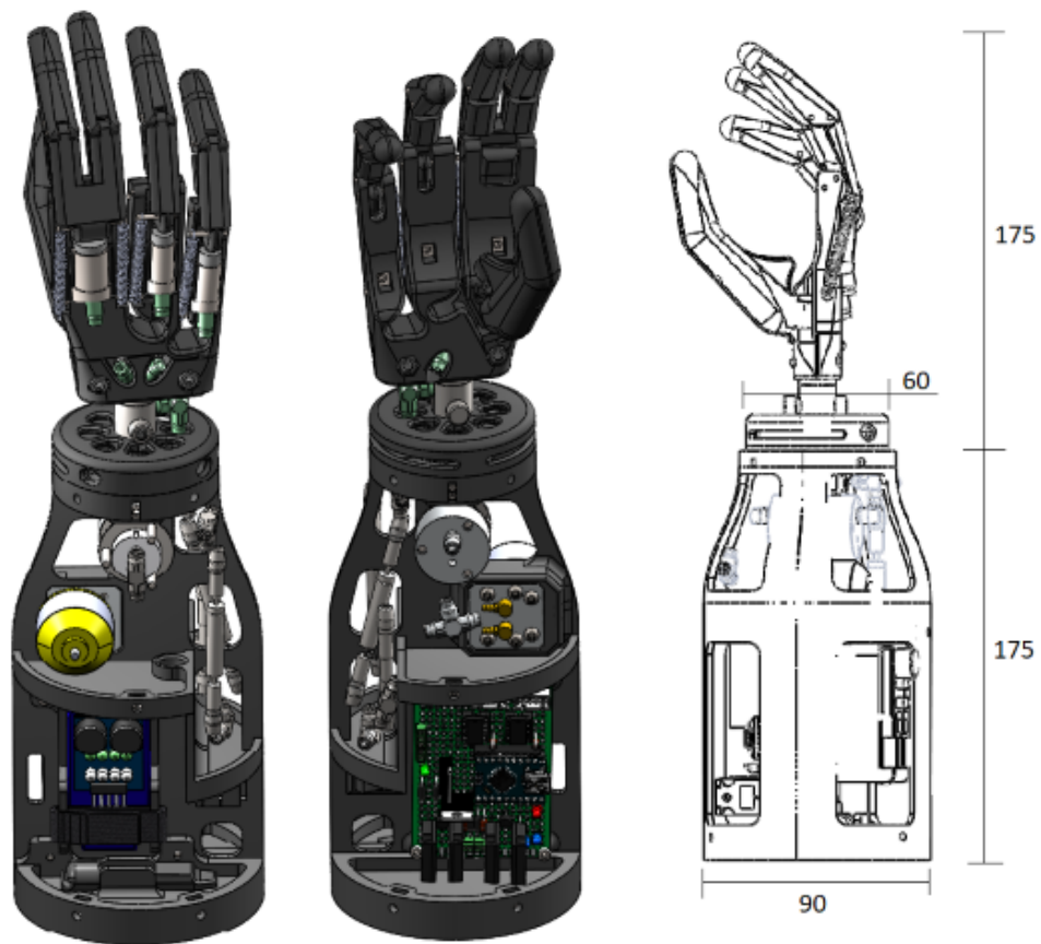
Fig. 75. Mechanical concept 4: Plate structure
