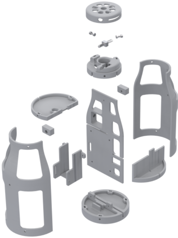
Fig. 13. An exploded view of the structure. The middle plate holds the components and connects to the wrist and the bottom disk. The two outer shells provide a stable structure and protect the inside components. The wrist mechanism, on top, consists of two circular components that slide into each other, with the spring loaded mechanism in between. The top part is connected to the hand and the bottom part to the rest of the structure. The slots in both parts allow hydraulic and electric cables to pass through.
