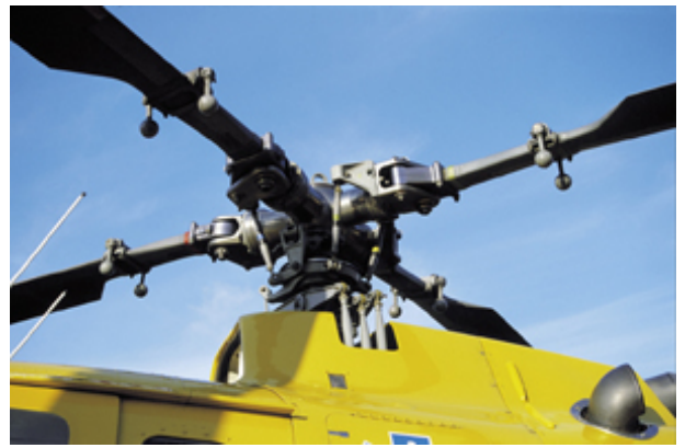
The blade’s flapping motion, lead-lag motion, and change of pitch are all made possible by hinges built into the rotor head, or in more recent types of helicopter, by flexible structural elements.
