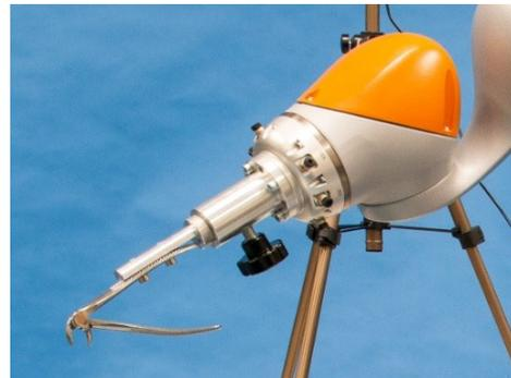
Fig. 4: Holding device for dental forceps.
