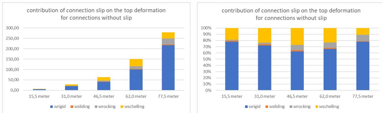
Figure 42, contribution of connection slip on the top deformation without initial slip
