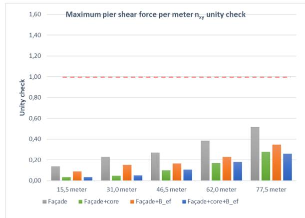
Figure 56, shear forces per meter on the piers in the façade for different models with additional components
