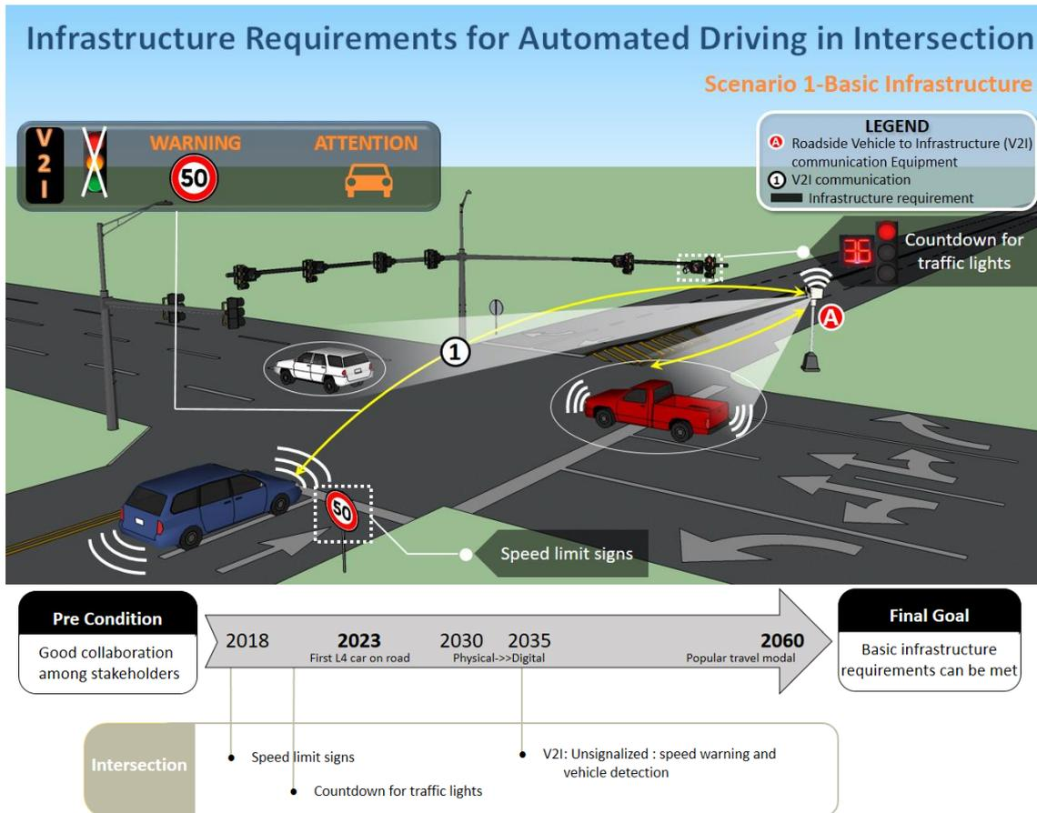
Figure 7.5 Infrastructure Requirements of Intersection in Scenario 1 (own illustration)
