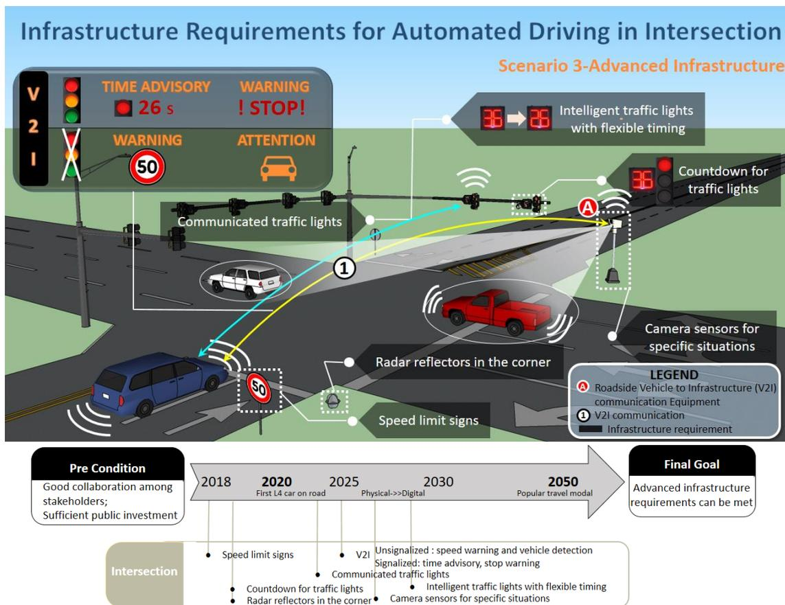
Figure 7. 10 Infrastructure Requirements of Intersection in Scenario 3 (own illustration)
