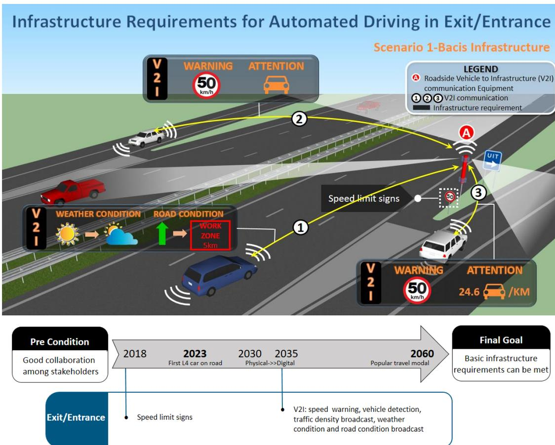
Figure 7. 4 Infrastructure Requirements of Motorway Exit/Entrance in Scenario 1 (own illustration)
