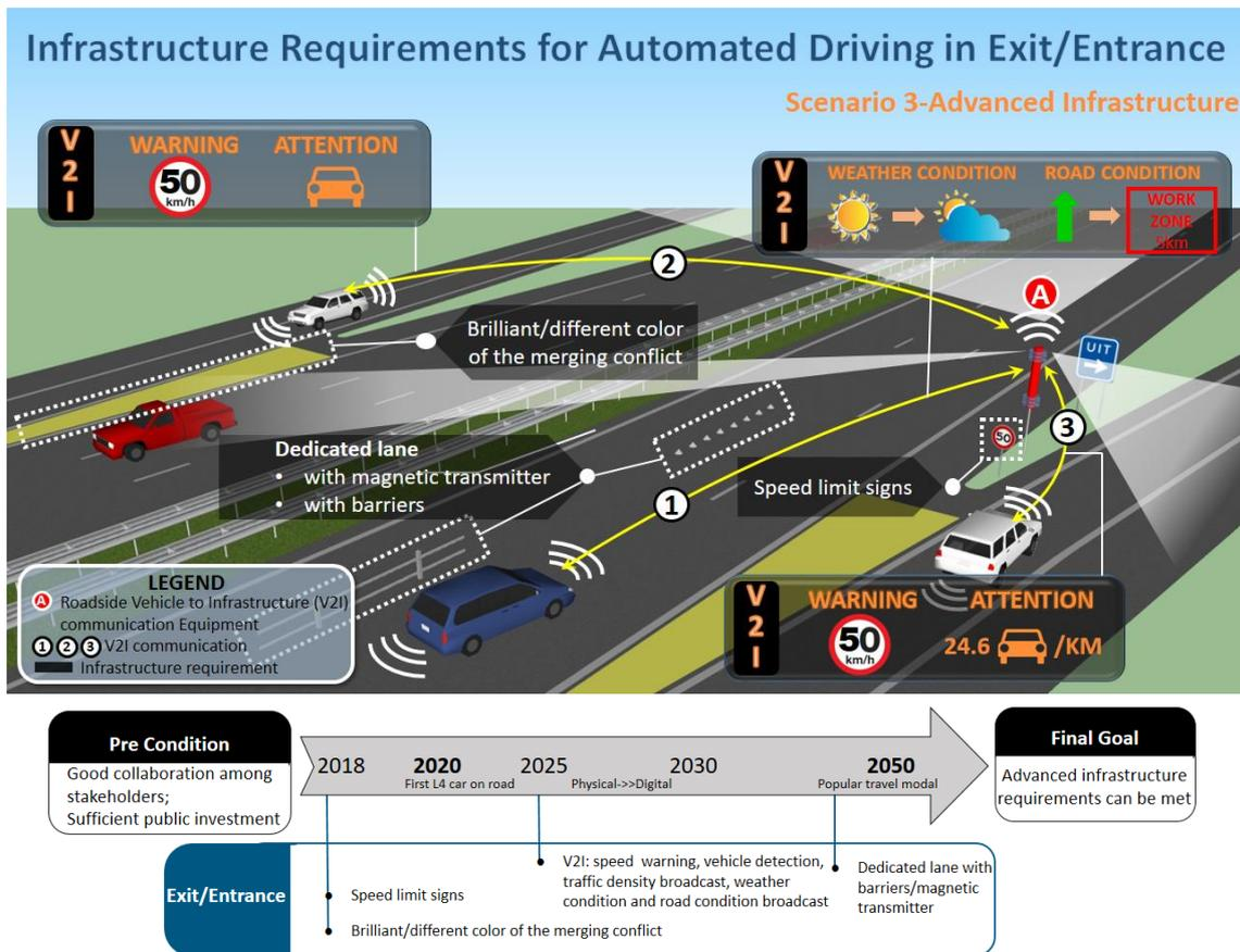
Figure 7.9 Infrastructure Requirements of Motorway Exit/Entrance in Scenario 3 (own illustration)
