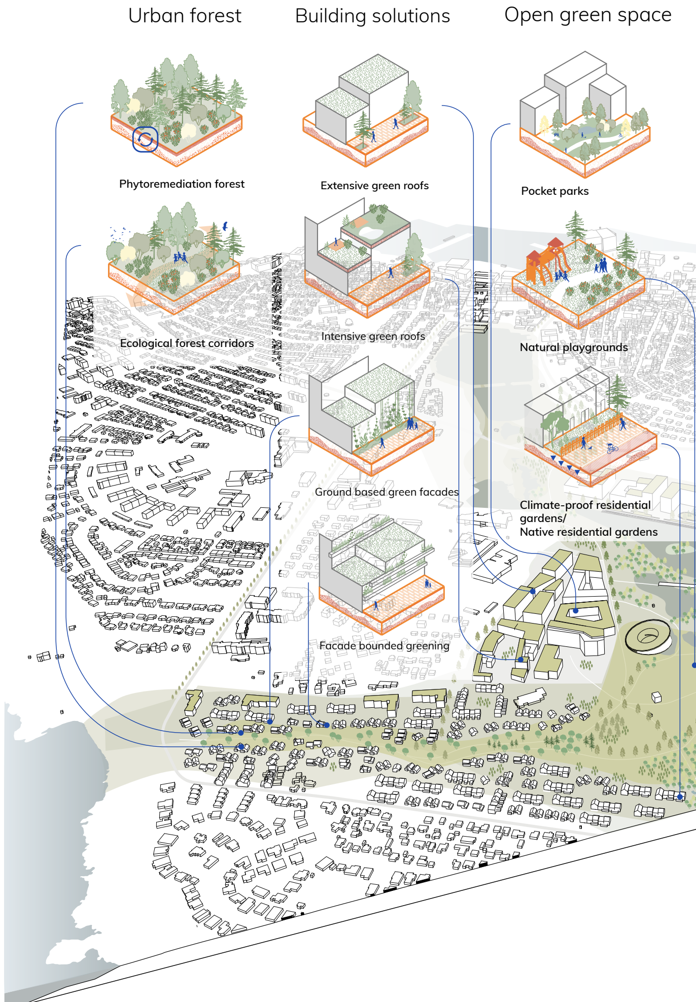
Figure 49: Axonometric of the blue-green network. Toolbox was developed to demonstrate the application of principles derived from nature based solutions and sponge-city principles
