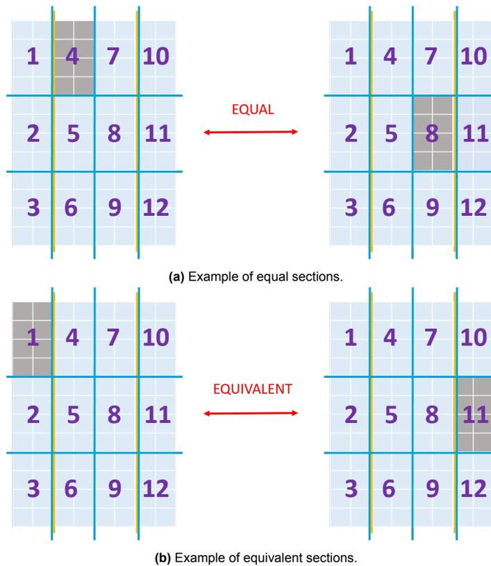
**Figure 4.11:** Examples showing equal vs equivalent sections in 96 cell module (12 rows x 8 columns, 3 bypass diodes in a [2 4 2] configuration).
