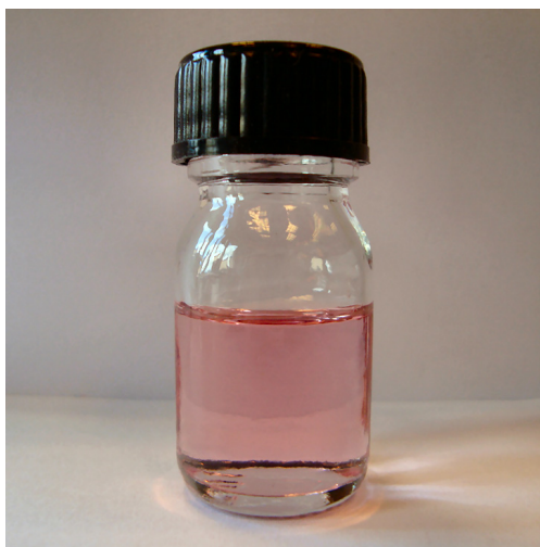
Fig. 6.2. Photo showing the typical colour obtained for the Au colloidal solutions by electro spraying into a reductive-surfactant solution (i.e. DDAM dissolved into cyclohexane).
