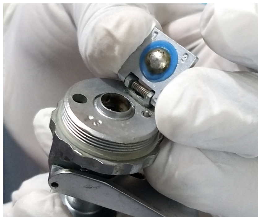
Fig 2.2.2 Dismantled Trocar Trapdoor spring
