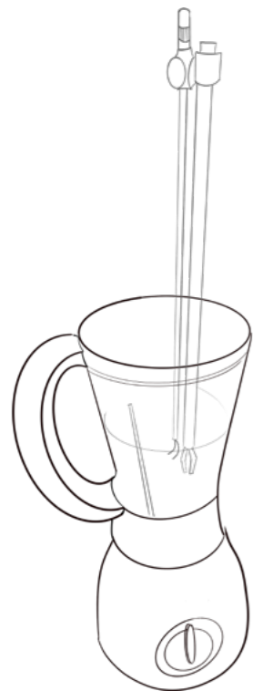
Testing the action of the circular flow of water on soiled laparoscopic instruments.
