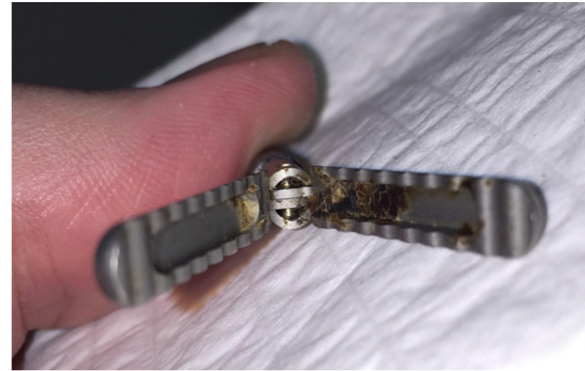
Fig 2.4.4 Traces of bioburden present on the laparoscopic grasper post sterilization.
