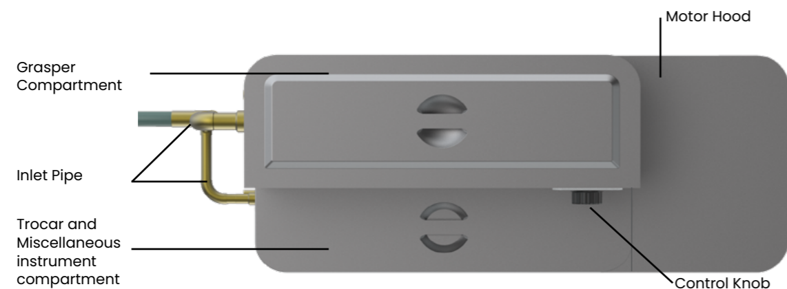
Fig 7.12 Top elevation of the mechanical washer body
