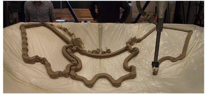
Fig. 17. Printing of the first prototype.
