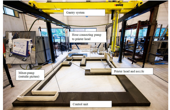
Fig. 3. 4 DOF Concrete Printer used at TU Eindhoven. Source: Bos et al. [7].
