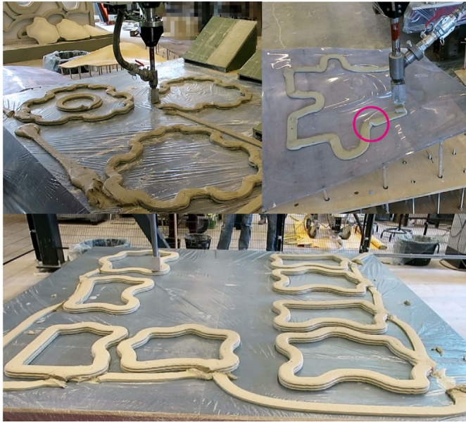
Fig. 11. Initial printing tests. [Left] Flat Geometry with 80 mm radius [right] 100 mm radius on flexible mould [bottom] flat with varying radii.
