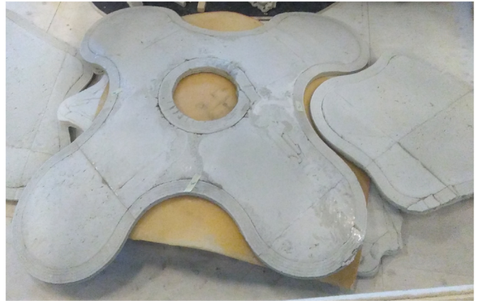
Fig. 21. Demolded final pavilion.
