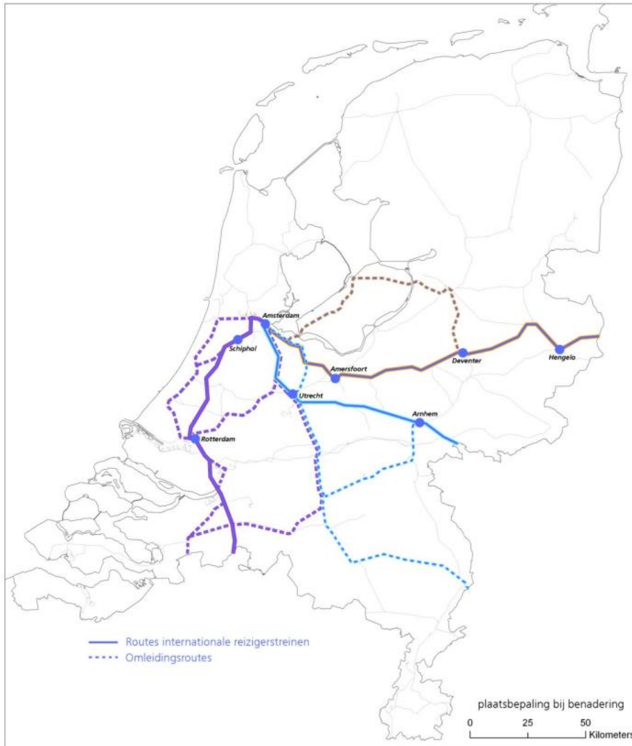
Figure 3.6: Rerouting options for international trains (ProRail, 2014).
