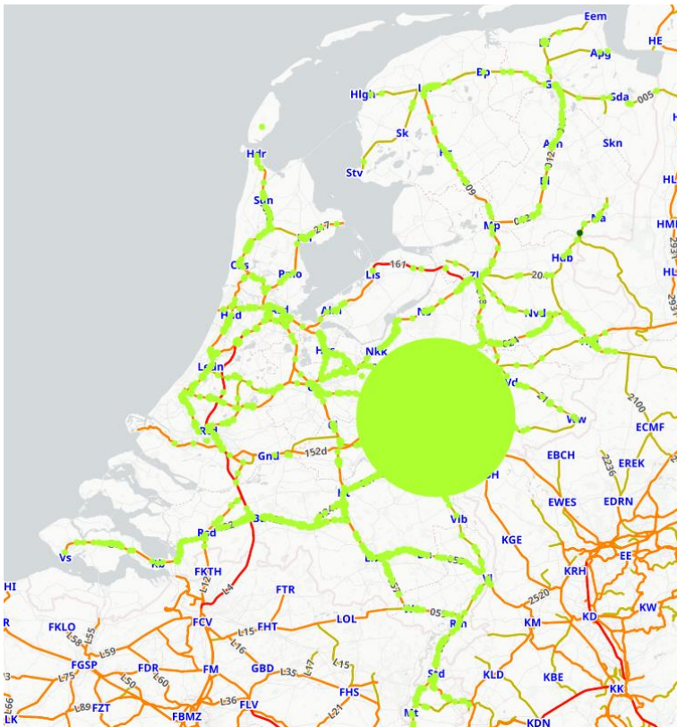
Figure B.12: Collision with a person with colour based on TIS code and radius based on occurrence.
