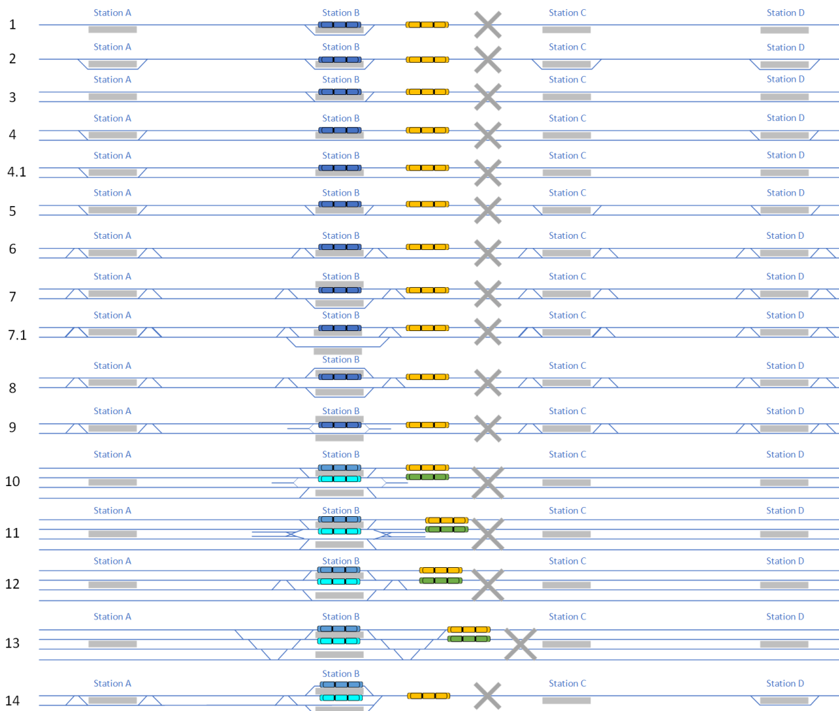
Figure 6.7: Tracks that are blocked during disruptions.
