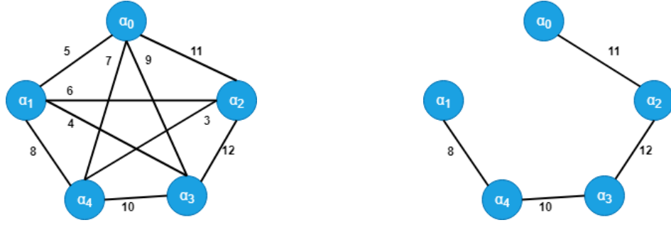
(a) The initial constraint-graph with 5 agents and 10 edges. (b) The resulting MST after applying the Kruskal's algorithm.
