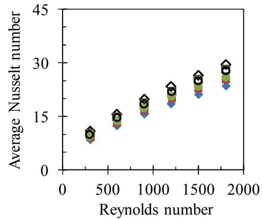
Figure 5. The relationship between  $Re$  and  $Nu_m$  when the thickness of the panel is 0.25 mm and the span of the brazing is 10 mm.
