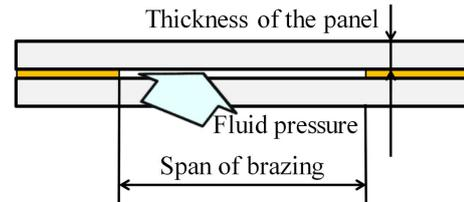
Table 2. Shape of each type of the test duct.
