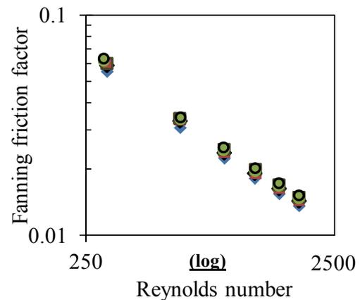
Figure 6. The relationship between  $Re$  and  $C_f$  when the thickness of the panel is 0.25 mm and the span of the brazing is 10 mm.
