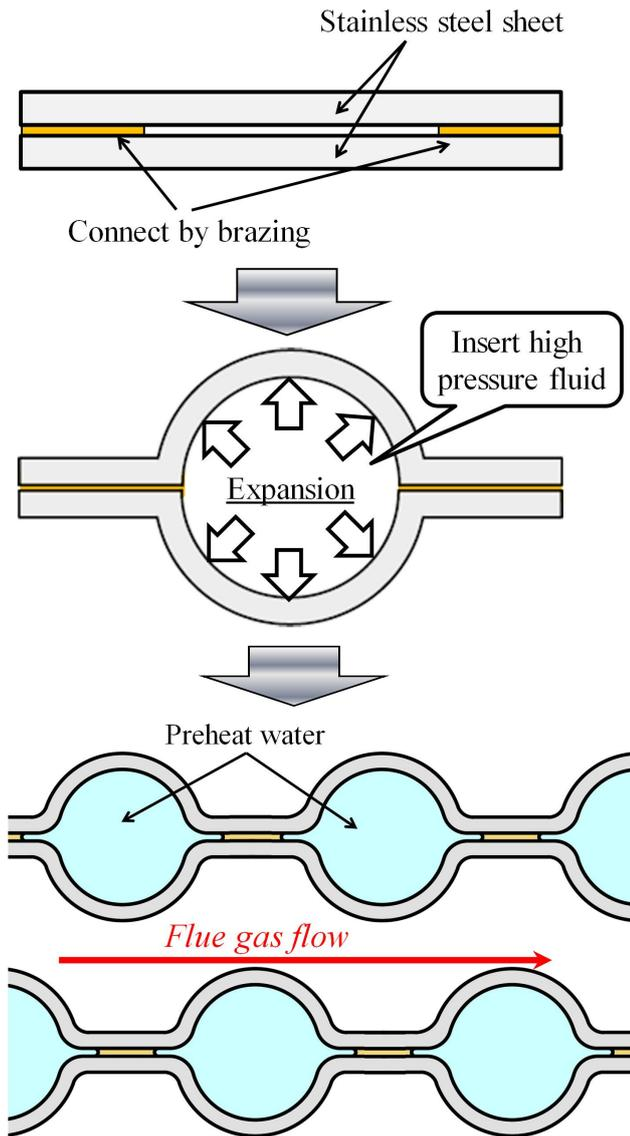
Figure 3. Image of how to make the heat exchange part.
