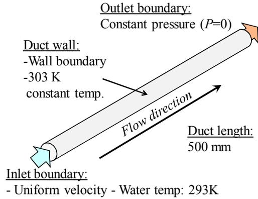
Figure 4. Analytical model and boundary conditions.
