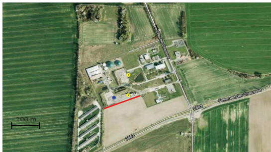
Figure 1 Satellite view of the injection site. The injection well is depicted in blue, observation wells in yellow and TNO's permanent surface receivers in red.
