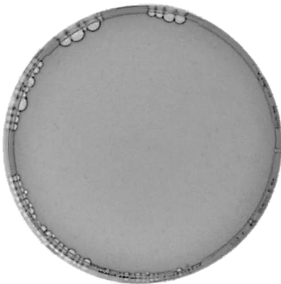
Green-Red sensor Under red light (650 nm) 0.026 W/m 2 , 24 hours
