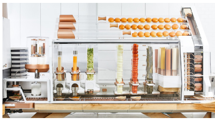
Figure 8 A transparent cooking robot which can make burgers from artisanal ingredients and is able to slice, grate, toast, season, grill and customize a burger freshly when ordered. Creator's Automatic Burger Cooking Machine, California, 2018.
