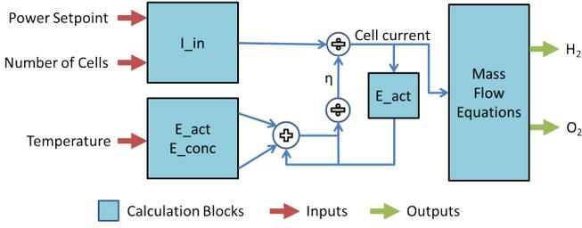
Fig. 1: electrolyzer Model
