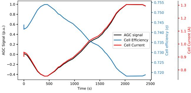
Fig. 3: electrolyzer cell performance given the AGC signal.
