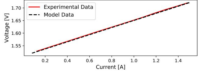
Fig. 2: Validation of the PEM electrolyzer cell model.
