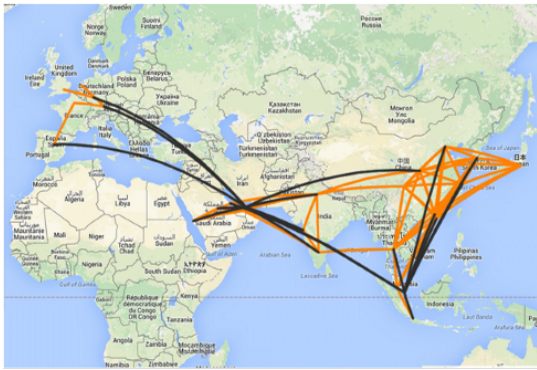
(a) Cost optimized network structure A for a given number of nodes and demand, solely considering fuel burn costs [37]
