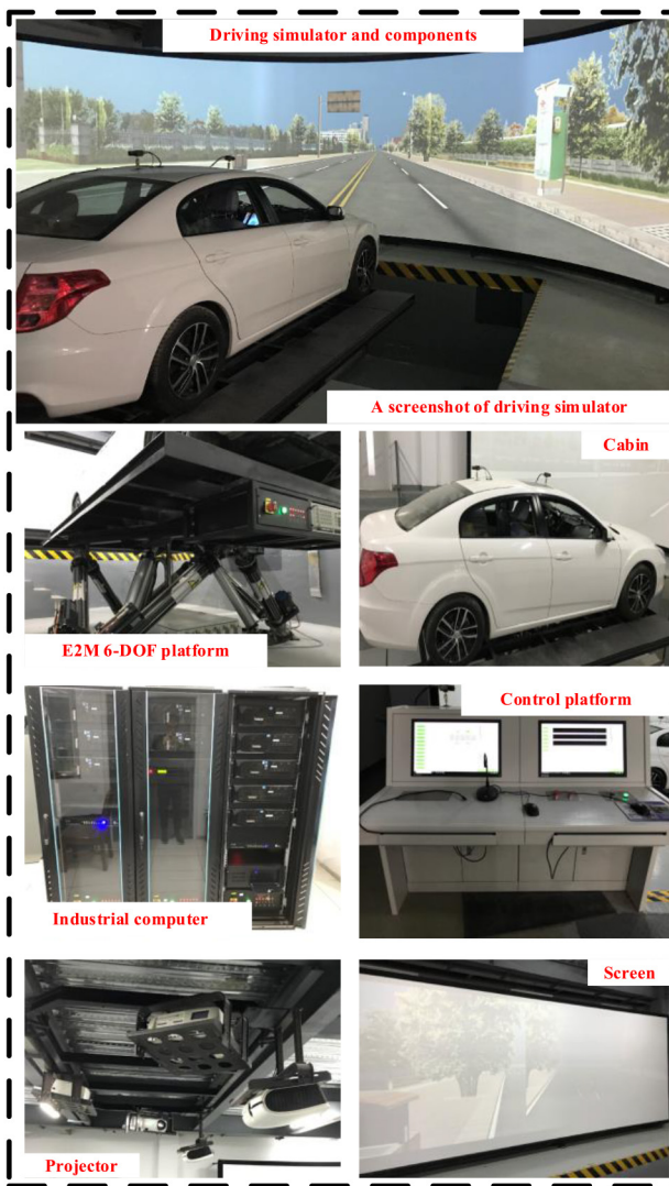
Fig. 4. Driving simulator and components.
