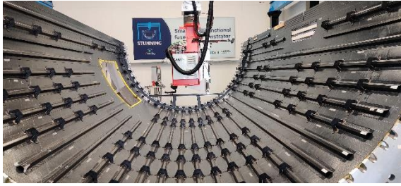
Fig. 9: Welding EEF in the CTS configuration being positioned over a clip to skin weld location on the lower shell of the fuselage demonstrator.
