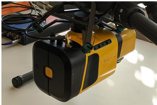
**Figure 6.16:** Setup with green dampers and untight tie wraps.
