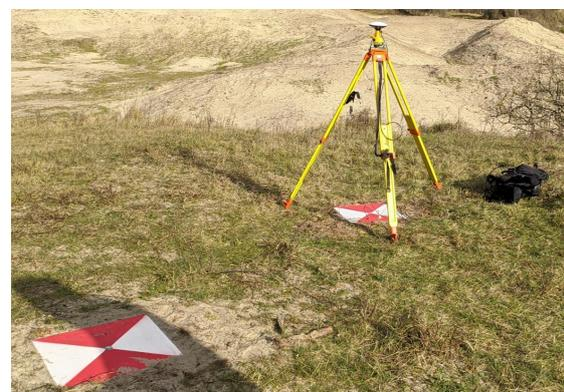
**Figure 6.2:** Picture of target 5 and 6. Target 6 has the GNSS reference station positioned on top. This picture was taken on a different date than the point cloud acquisition.
