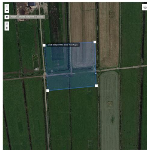
Figure 4.3: Selecting region of interest in the DJI flight planner tool.
