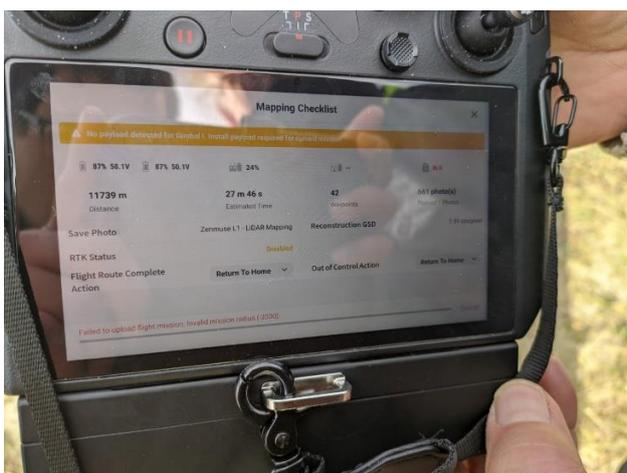
Figure 6: Invalid mission radius error on the UAV controller.
