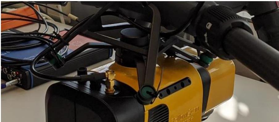
*Figure 2: Shows the dampers of the DJI SkyPort.*
