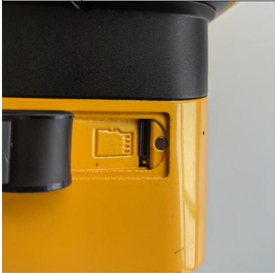
Figure 7: Indication how micro-SD card should be connected.
