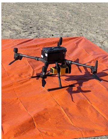
Figure 3.1: Complete LiDAR UAV system.
