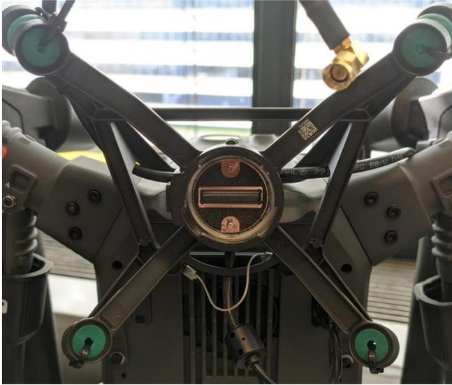
Figure 8: DJI SkyPort in correct position.
