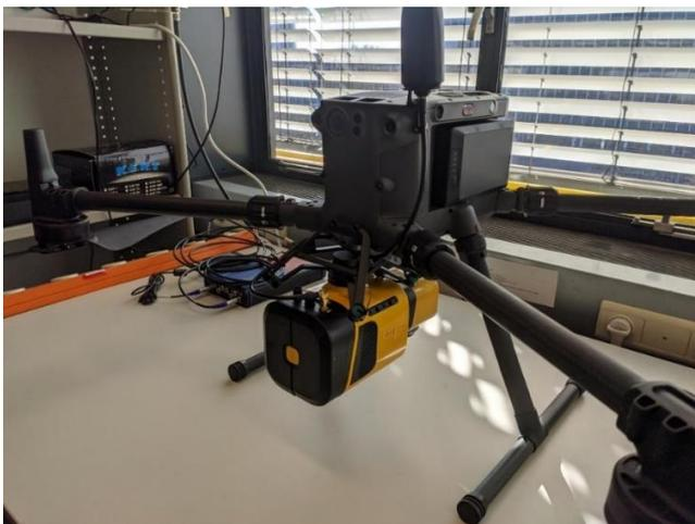
*Figure 1: DJI Matrice 300 RTK with Yellowscan Mapper+.*
