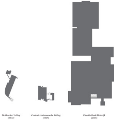
Figure 8 Size comparison of dutch auction houses built in different periods. The grey filled spaces are for product storage and logistics, whereas the actual auction room is marked as white. The shrink of auction rooms' percentage is a result of improvement on infrastructure so that the auction house can handle more products and technology that automatic conveyor belts and information systems allow multiple auctions to take place simultaneously.
