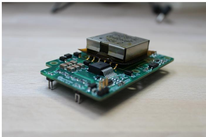
Figure A.5: The illustration of the Flyback Converter v.1.
