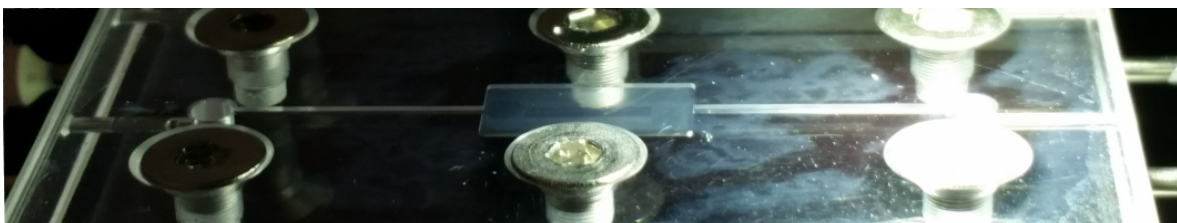
Figure B-4: Picture showing the milky/blueish haze of insulin that has leaked from the test-conduit into the capillary space between the two PMMA slabs and PVC foil.
