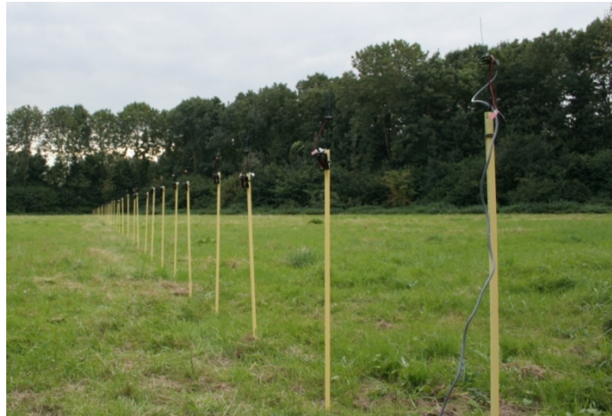
Figure 4-1. The right most pole holds the transmitter, which is connected via a USB cable to a laptop. 30 receivers are positioned along a line of 100 meters.
