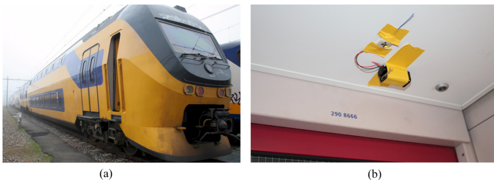
Figure 5-1. (a) V-IRM2; (b) node and battery attached to the interior with tape.
