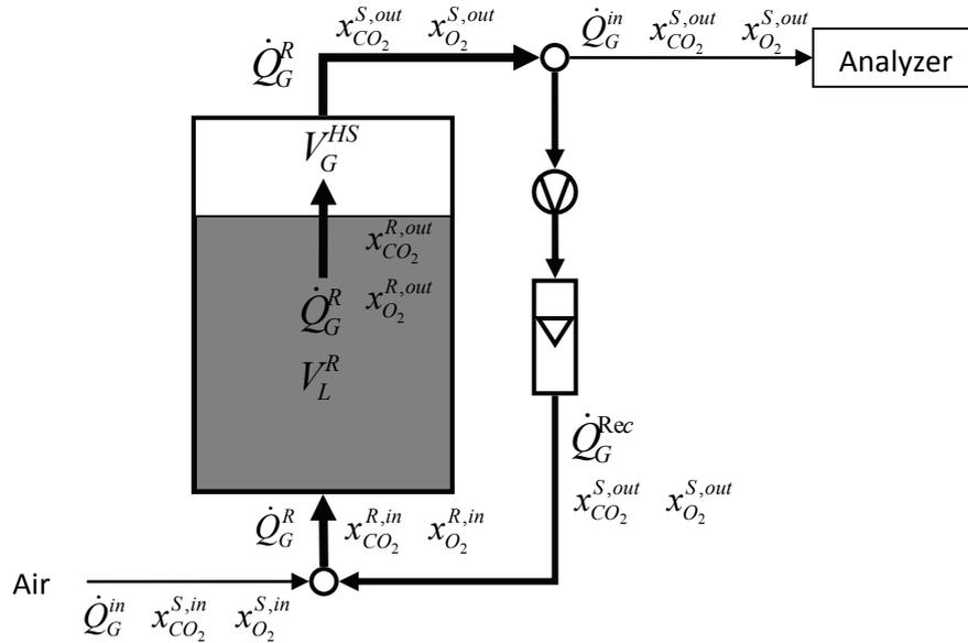
**Figure 2.1.** Scheme of the off-gas recycling set-up. S and R indicate boundaries for mass balances for calculating oxygen and carbon dioxide transfer rates.
