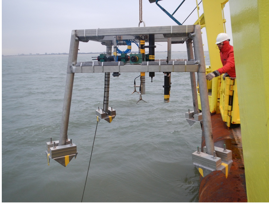
Figure 2: Deployment of the NEMO lander.
