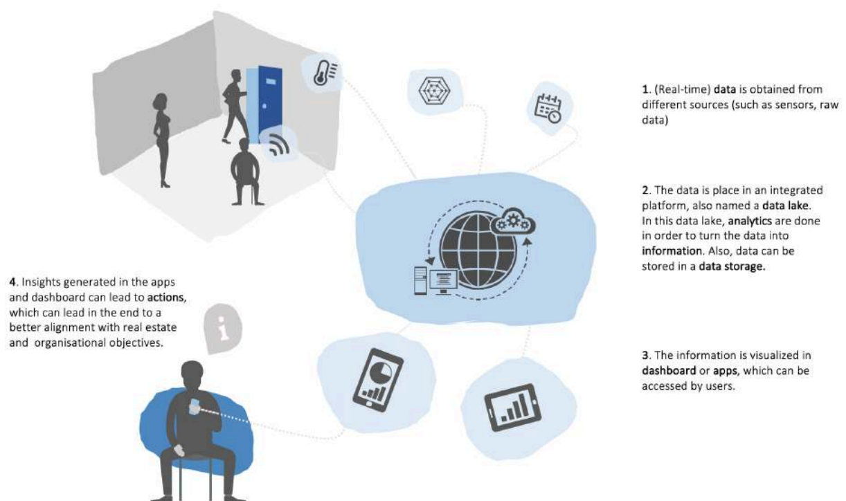
Figure a. Visualization of the smart tool principle (own illustration)
