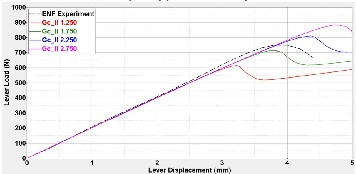
(b) Load-Displacement graph of 3D simulations 25 through 28.
