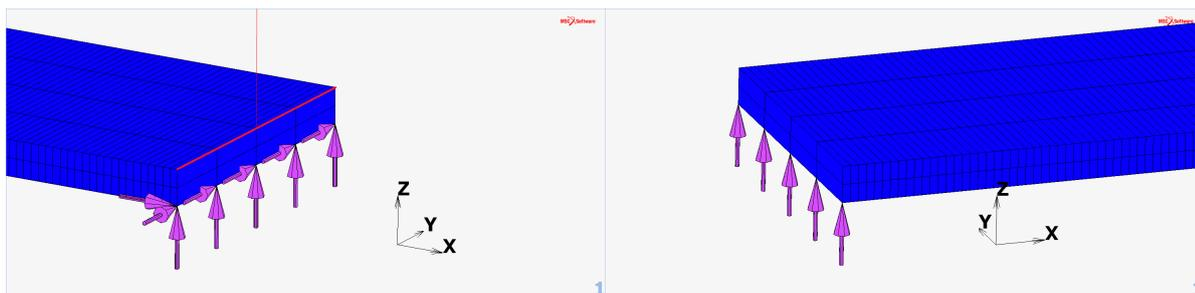
(b) Bottom corner nodes at start of initial crack fixed in x-, y- and z-direction.
