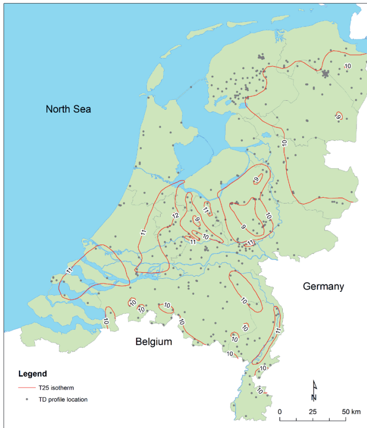
Figure 2.1: Isotherms [°C] at 25 m below ground surface, based on Van Dalfsen (1983), with locations of TD-profiles measured by Van Dalfsen.
