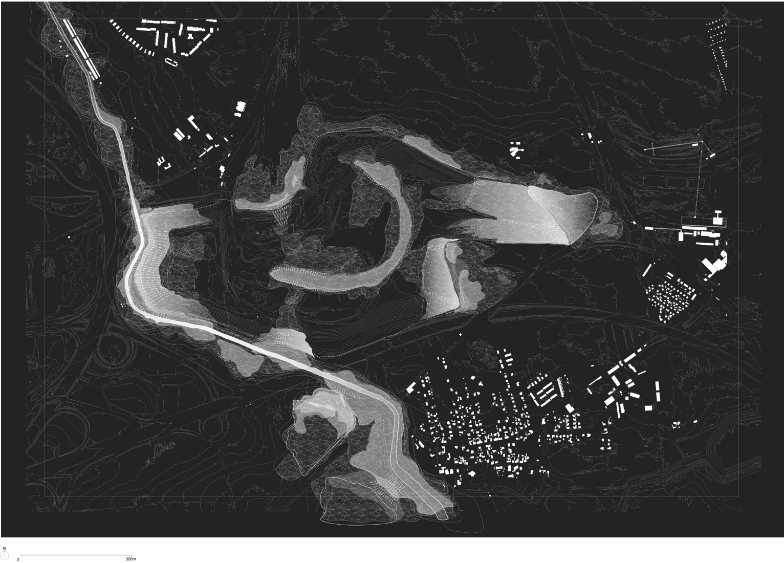
Figure 20 | Toxic run-off water mapping and Acide mine draining prone areas - bright white patterns reflects the water runoff from the heap which directly affects nearby water bodies like Kłodnica river, Marshlands and the Sedimentation lake
