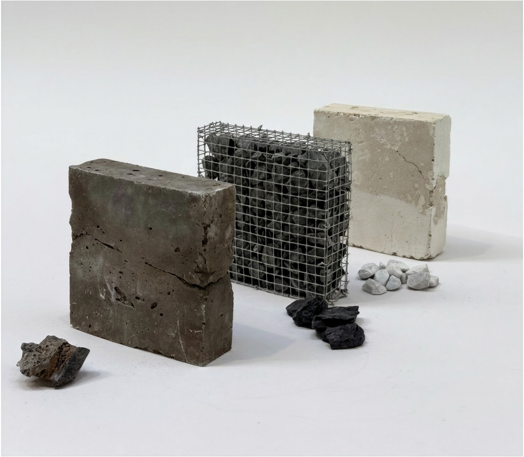
Figure 38 | Material exploration through model making Three types of walls were constructed using materials extracted during the site visit. From the front, these include: limestone with iron staining, a gabion wall infilled with a mixture of rock and coal, and lastly, a concrete wall made from crushed concrete debris.
