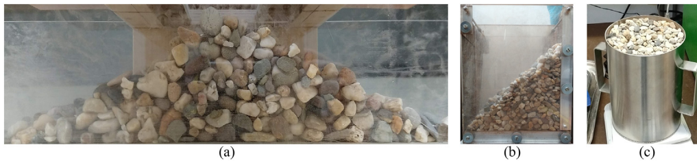
Fig. 1. Laboratory scale tests (a) Pile forming test (b) Ledge test (c) Bulk density test.
